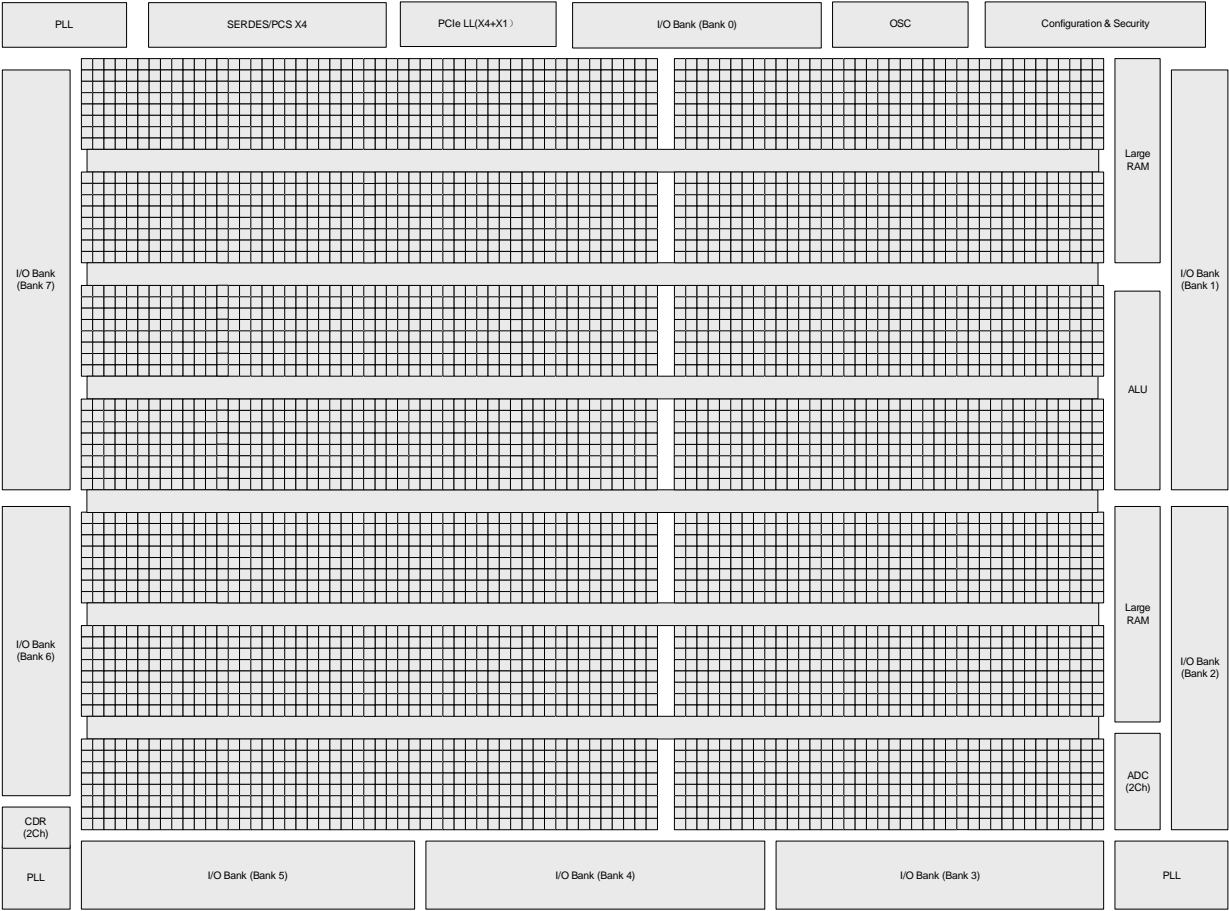
Figure 2.1. Simplified Block Diagram, LFCPNX-50 Device (Top Level)
