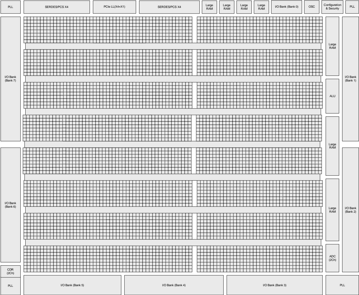
Figure 2.2. Simplified Block Diagram, LFCPNX-100 Device (Top Level)
