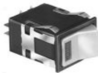
AML36 Series Rocker Switch, SPST, 2 position, Silver Contacts, 0.187 in x 0.02 in (Solder or Quick-Connect) With Isolated Lamp Circuit, 1 Lamp Circuit, Rectangle, Snap-in Panel
