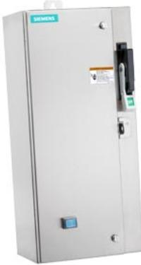
Non-reversing motor starter, Size 1, Three phase full voltage, Solid-state overload relay, OLR amp range 0.75-3.4A, 110V 50Hz / 120V 60Hz coil, Combination type, 30A fusible disconnect, 30A/250V fuse clip, Encl NEMA type 4X 304 S-Steel, Water/dust tight noncorrosive, Standard width enclosure
