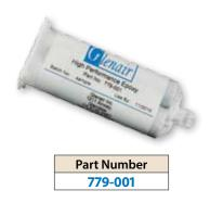
High performance flexible two part thermoset epoxy provides high strength flexible bond from -55° to 150°C. 50 ml duo syringe fits standard dispensing guns. Use with square green mixing nozzle sold separately. 12 hour cure time at 20°C, 1 hour at 85°C, 30 minutes at 150°C. Apply to inside of boot with wooden spatula. 18 month shelf life.
