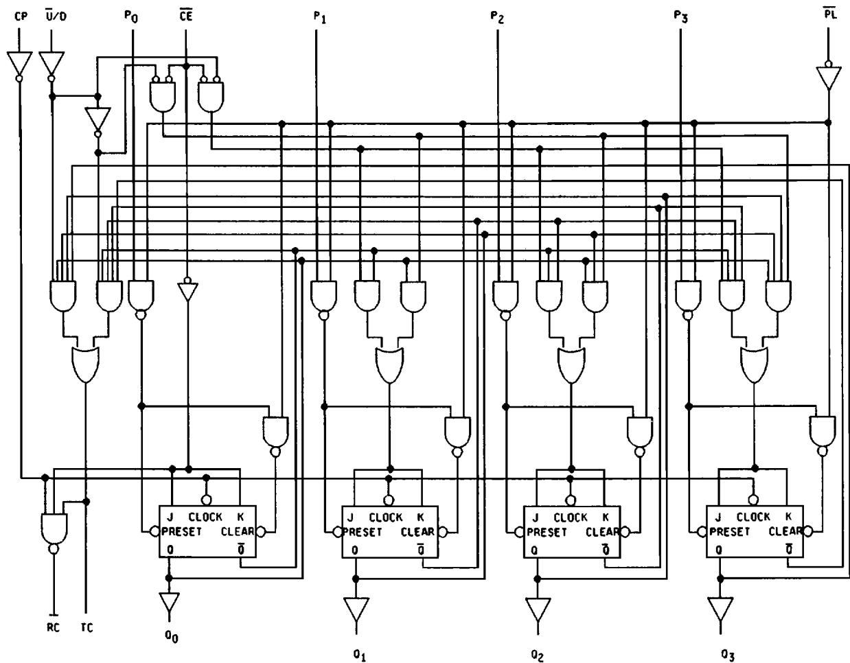
FIGURE 3. Logic diagram.
