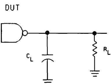
FIGURE 4. Test circuit and switching waveforms.
