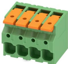
Printed circuit board terminal, nominal current: 41 A, rated voltage (III/2): 1000 V, nominal cross section: 6 mm<sup>2</sup>, number of potentials: 4, number of rows: 1, number of positions per row: 4, product range: LPT 6/, pitch: 7.5 mm, connection method: Lever Push-in connection, mounting: Wave soldering, conductor/PCB connection direction: 0 °, color: green, Pin layout: Zigzag pinning W, Solder pin [P]: 3.6 mm, type of packaging: packed in cardboard
