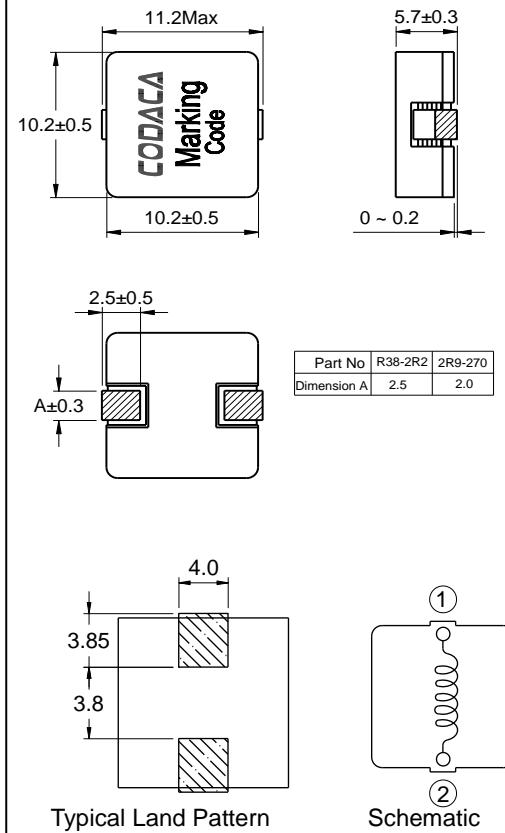
All data is tested on 25°C ambient temperature
