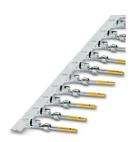
Crimp contact, Pin, rolled, Taped product, number of pieces per reel: 500, contact diameter: 1 mm, crimp range: 0.08  $\rm mm^2$  ... 0.22  $\rm mm^2$
