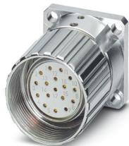
M23, Device connector front mounting with knurled nut, series: RC, straight, shielded: yes, Screw locking mechanism, No. of pos.: 12, Direction of rotation: Counter direction, contact connection type: Socket, Solder cup, Radial O-ring, 4x Ø 3.2, coding: N
