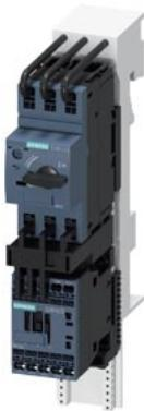
Load feeder fuseless, Direct-on-line starting 400 V AC, Size S00 0.35...0.50 A 24 V DC Spring-type terminal for 60 mm busbar systems (also fulfills type of coordination 1) Type of coordination 2,  $I_q = 150 \text{ kA}$  1 NO (contactor)
