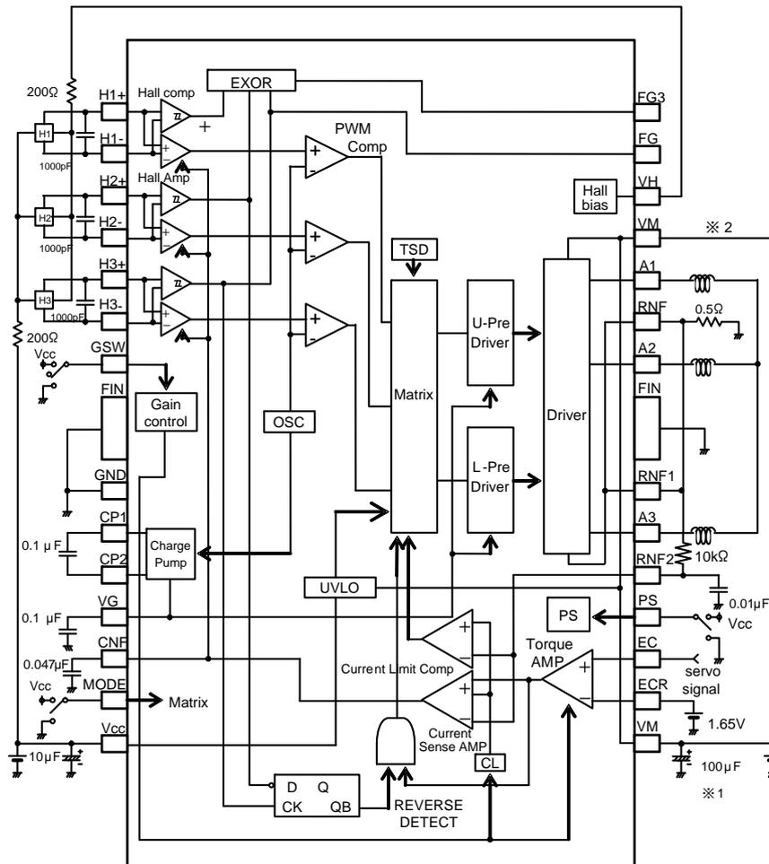
※ 1 Set capacitor between VM and GND, close as possible to the IC.
