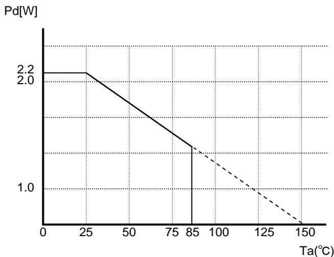
Fig.7 Power Dissipation Reduction (BA6664FM, BD6671FM)
