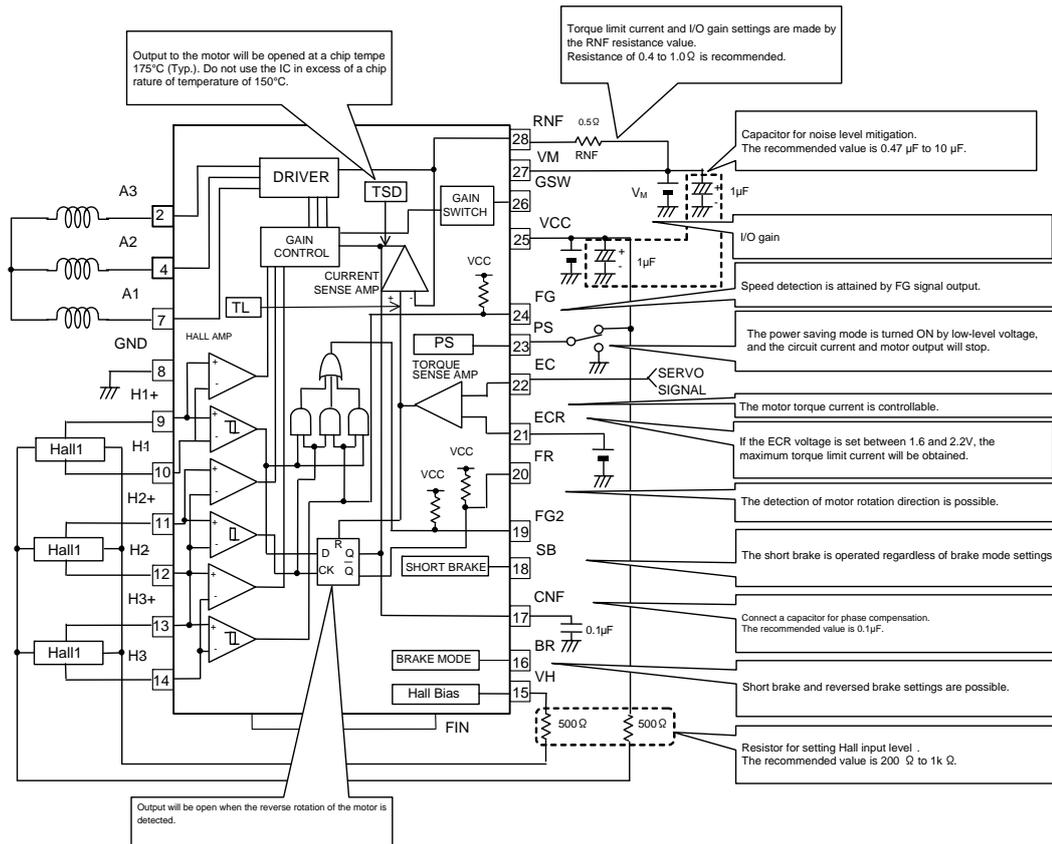
Fig.6 BA6664FM Block Diagram
