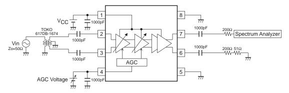
Output Voltage is divided by  $50\Omega$  /  $(200+50)\Omega$
