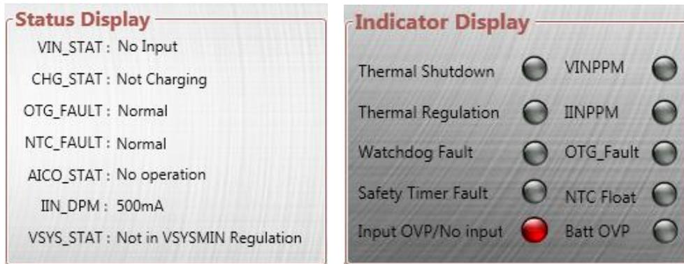
**Figure 28: Monitoring the MP2723A Status and Faults**
