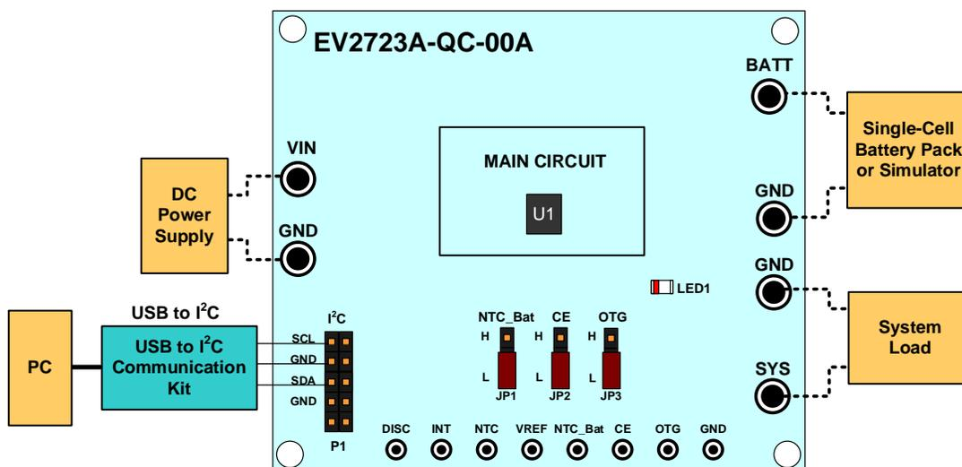
**Figure 2: Test Set-Up for the MP2723A**
