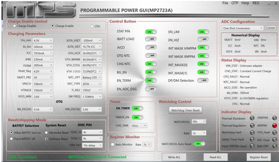
Figure 3: The MP2723A Evaluation Software
