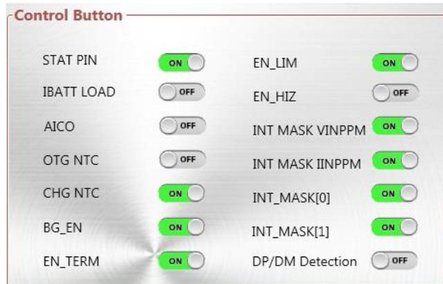
Figure 24: Adjustable Parameters for the MP2723A
