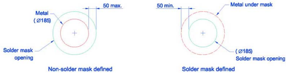
Solder mask detail (not to scale)
