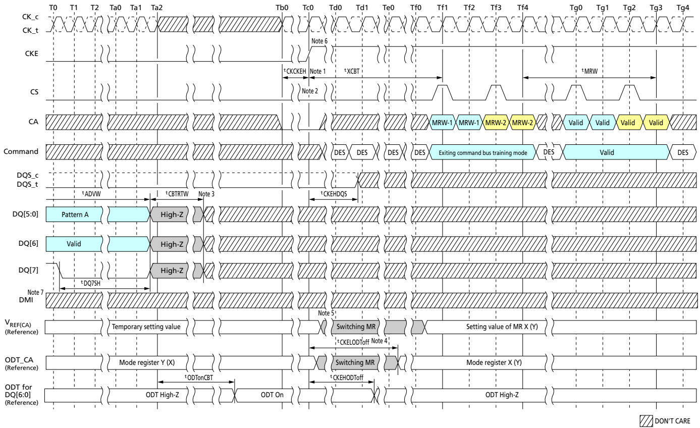
Figure 213: Exiting Command Bus Training Mode
