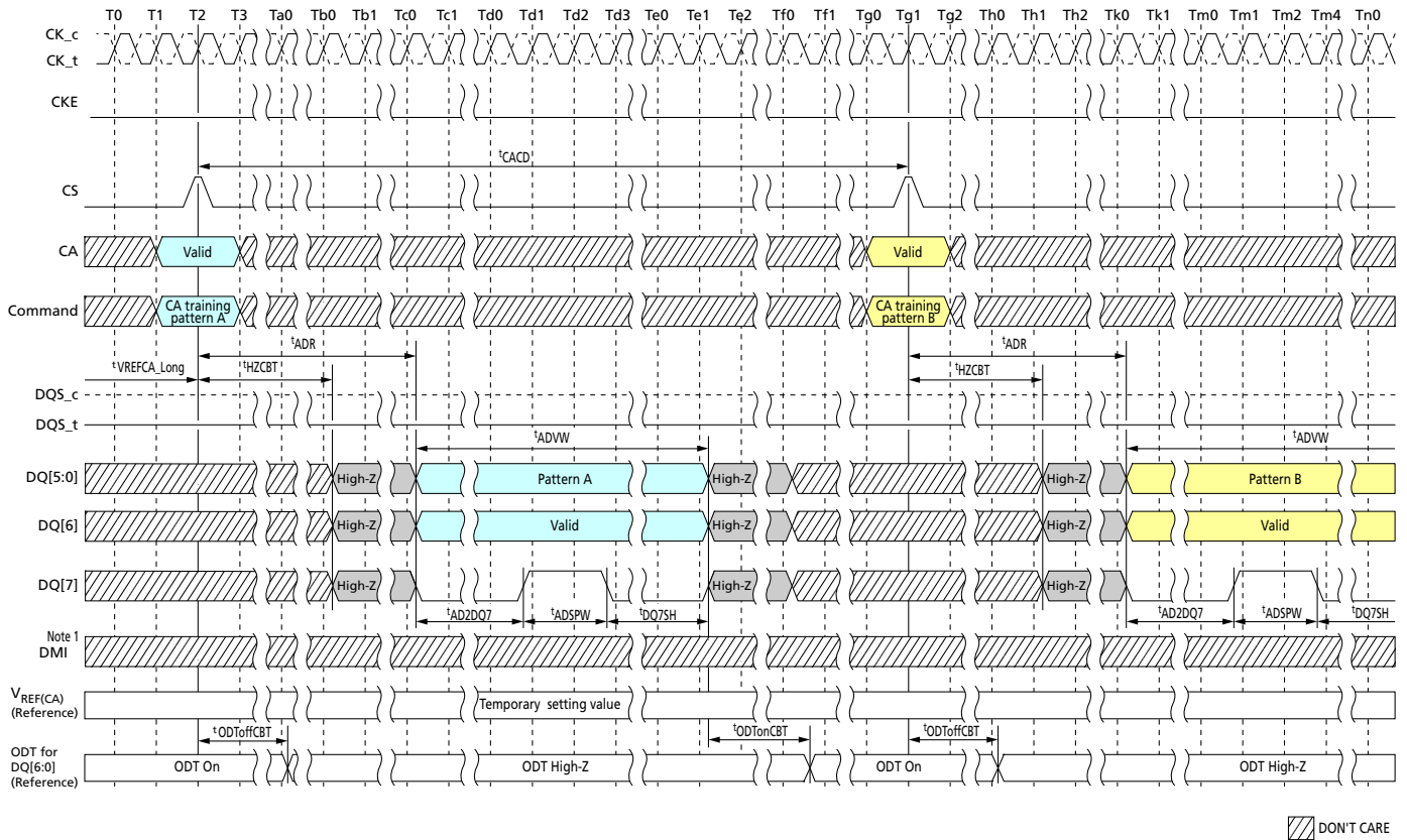
Figure 212: Consecutive CA Training Pattern Input/Output
