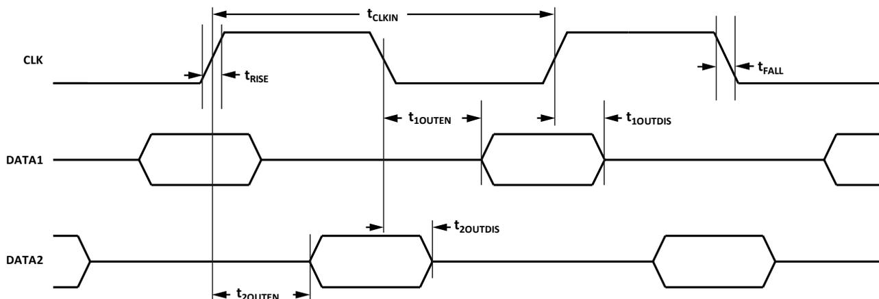
**Figure 1. Pulse Density Modulated Output Timing**
