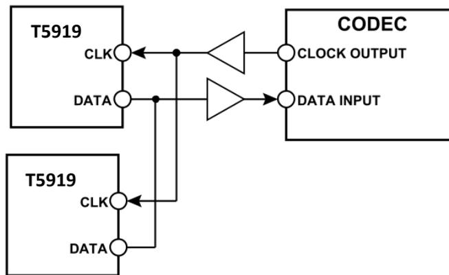
**Figure 14. Buffered Connections Between Stereo T5919s and a Codec**
