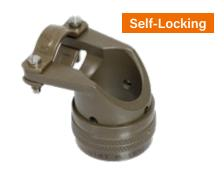
**Self-locking. Full radius saddles.** Open frame saddle clamp fits Series 806 MilAero connectors. Anti-decoupling mechanism provides audible detented coupling and prevents backoff under high vibration. Die cast saddle bars have self-locking stainless steel clinch nuts. Full radius saddles are intended to be fully closed (bottomed onto frame). Aluminum or stainless steel.
