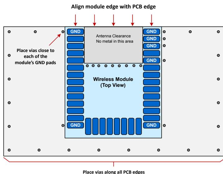
Figure 7.1. Recommended Layout for MGM240P Using Built-in Antenna
