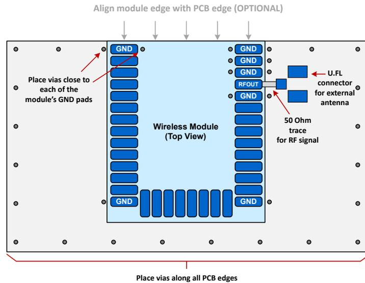
**Figure 7.2. Recommended Layout for MGM240P Using External Antenna**
