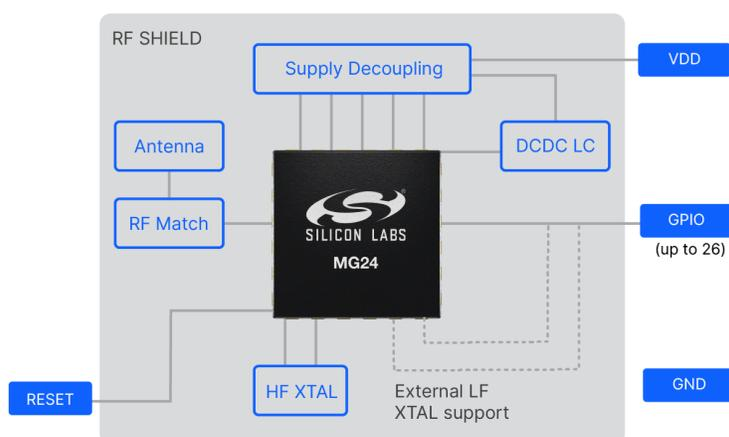
Figure 3.1. MGM240P Block Diagram - Built-in Antenna Variant
