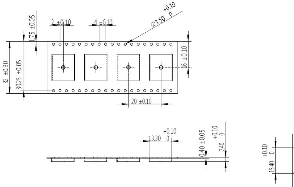
Figure 10.1. Carrier Tape Dimensions
