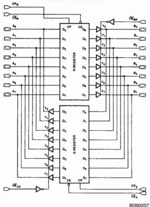
Note: The Am2953 provides inverting data output
