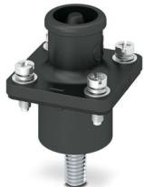
Connector, Range of articles: BPC, color: black, number of positions: 1, min. conductor cross section: 35 mm<sup>2</sup>, max. conductor cross section: 70 mm<sup>2</sup>, rated voltage: 1500, rated current: 250 A, Connection method: Screw/Solder connection, Contact connection type: Pin
