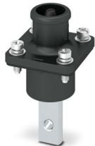
Connector, Range of articles: BPC, color: black, number of positions: 1, min. conductor cross section: 16 mm<sup>2</sup>, max. conductor cross section: 25 mm<sup>2</sup>, rated voltage: 1500, rated current: 120 A, Connection method: Screw connection, Contact connection type: Pin
