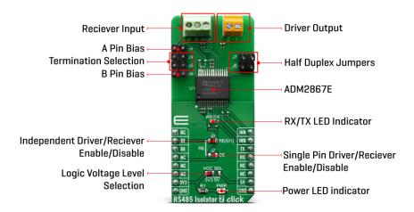
The integrated dc-to-dc converter is optimized to minimize radiated electromagnetic interference (EMI), and allows designers to meet the CISPR22/EN55022 Class B requirements on a 2-layer PCB.
