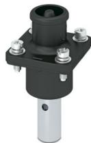
Connector, Range of articles: BPC, color: black, number of positions: 1, min. conductor cross section: 16 mm<sup>2</sup>, max. conductor cross section: 25 mm<sup>2</sup>, rated voltage: 1500, rated current: 120 A, Connection method: Crimp, Contact connection type: Pin
