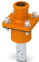
Connector, Range of articles: BPC, housing material: PA, color: orange, number of positions: 1, min. conductor cross section: 35 mm<sup>2</sup>, max. conductor cross section: 70 mm<sup>2</sup>, rated voltage: 1500, rated current: 250 A, Connection method: Screw/Solder connection, Contact connection type: Pin
