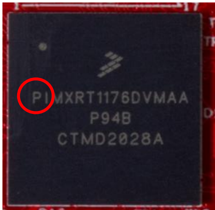
Figure 8 – Identifying Early Silicon Revision of the i.MX RT1176 (on rev PA4 and rev A Boards)
