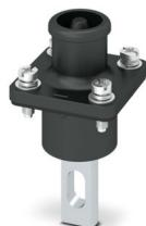
Connector, Range of articles: BPC, color: black, number of positions: 1, min. conductor cross section: 35 mm<sup>2</sup>, max. conductor cross section: 70 mm<sup>2</sup>, rated voltage: 1500, rated current: 250 A, Connection method: Screw/Solder connection, Contact connection type: Pin
