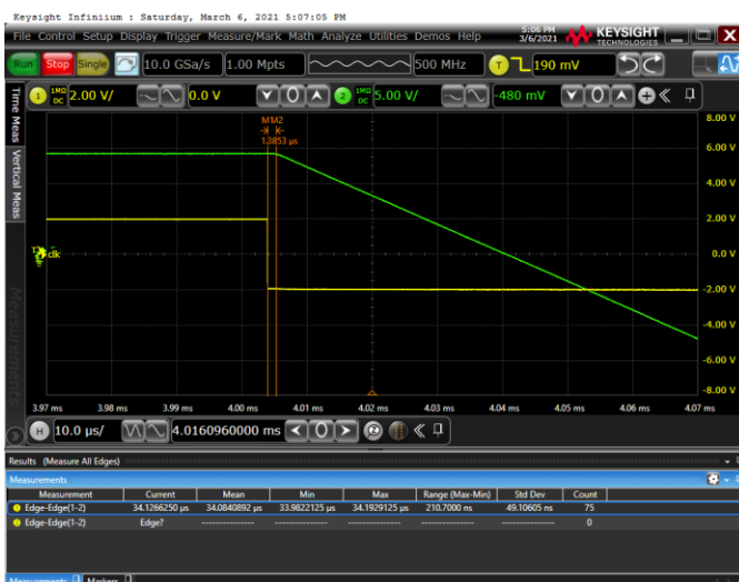
Time: 10μs/div, Measure Time: 1.4μs, G=11
