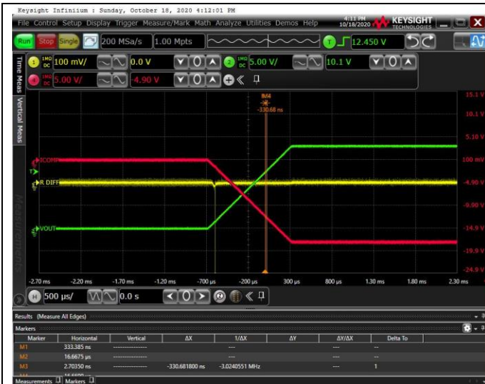
Figure 23. 1ms Power On and Off Time
