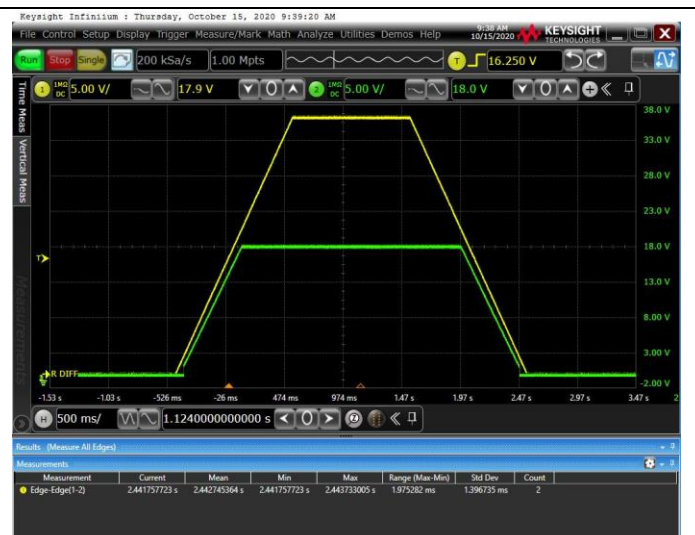
Figure 22. 1s Power On and Off Time
