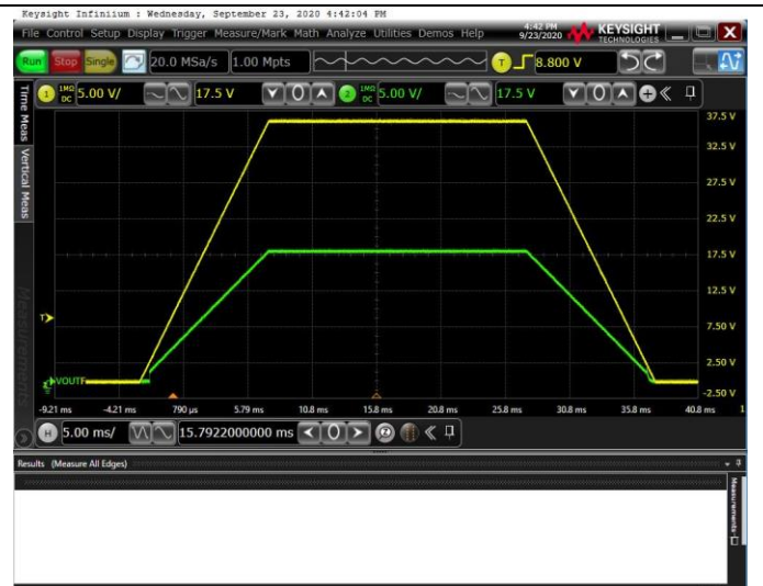
Figure 20. 10ms Power On and Off Time
