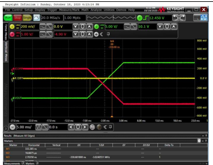
Figure 24. 10ms Power On and Off Time
