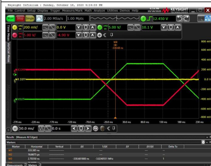
Figure 25. 100ms Power On and Off Time
