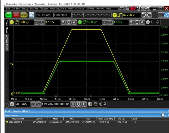
Figure 21. 100ms Power On and Off Time
