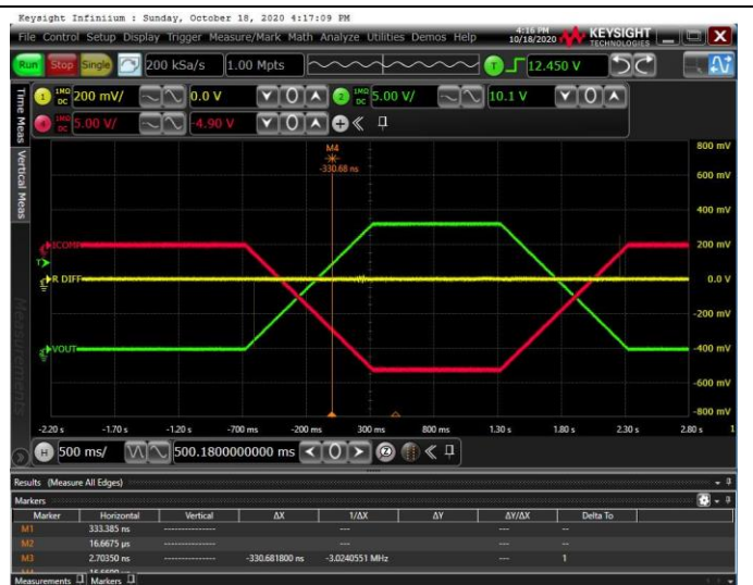
Figure 26. 1s Power On and Off Time
