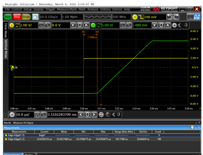
Time: 10μs/div, Measure Time: 7.8μs, G=11
