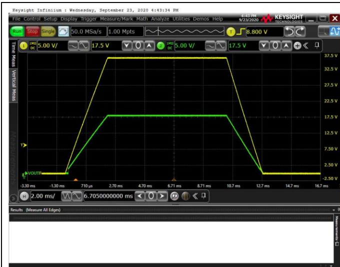
Figure 19. 2ms Power On and Off Time
