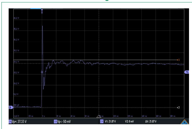
SC1122 IEC 61000 -4-2 +8 kV Contact ESD Clamping Voltage
