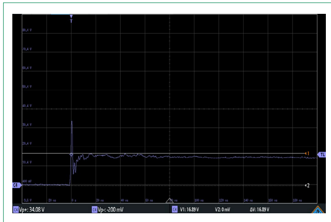
SC1115 IEC 61000 -4-2 +8 kV Contact ESD Clamping Voltage
