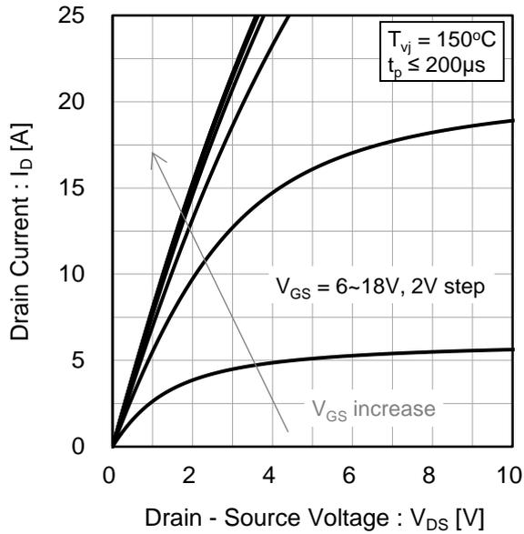
Fig.7  $T_{vj} = 150^{\circ}\text{C}$  3rd Quadrant Characteristics
