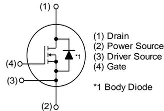
Please note Driver Source and Power Source are not exchangeable. Their exchange might lead to malfunction.
