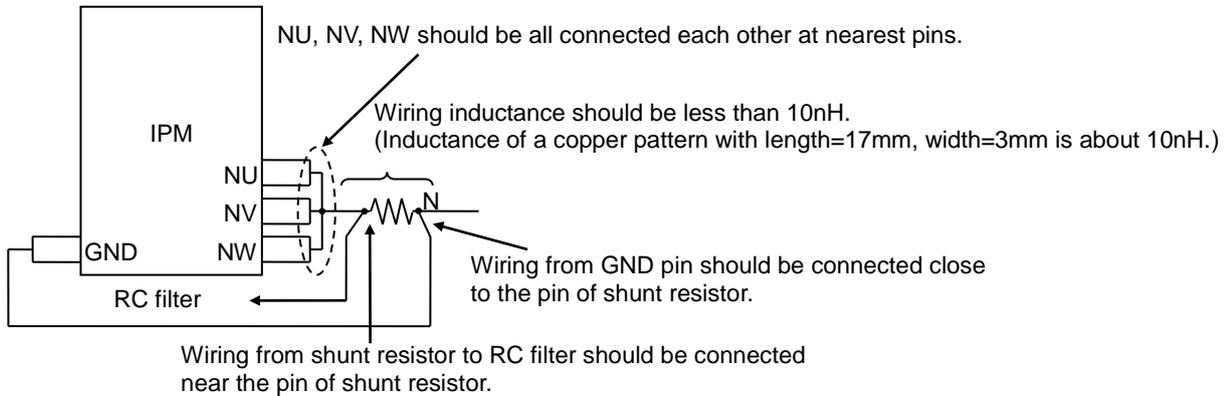
Low inductance shunt resistor like surface mounted (SMD) type is recommended.
