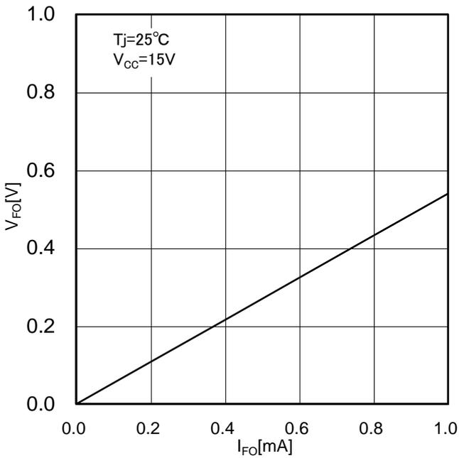
Figure 9.  $V_{FO}$  vs  $I_{FO}$
