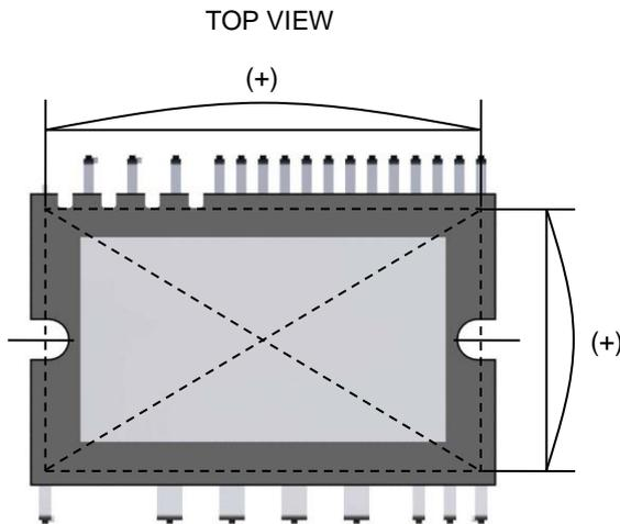
Figure 6-1. Measurement Point of Heat Sink Flatness
