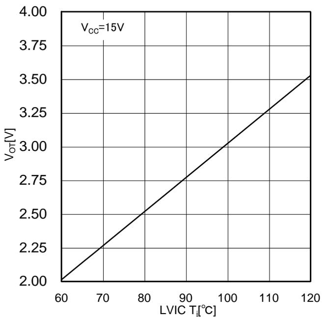
Figure 10.  $V_{OT}$  vs LVIC  $T_j$
