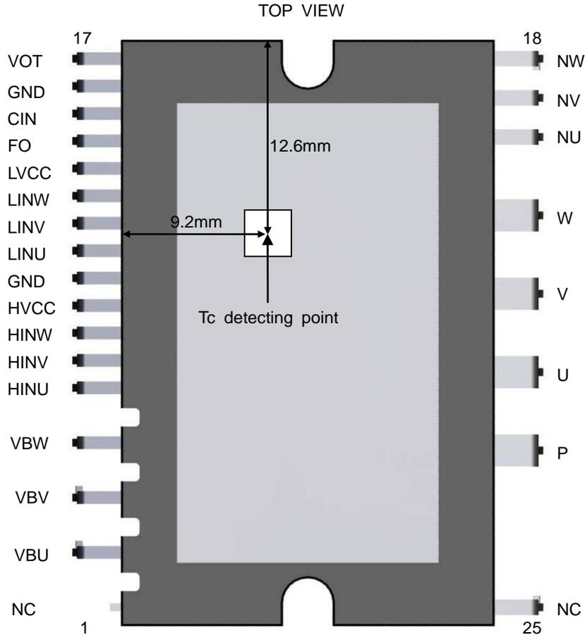
Figure 2. Pin Configuration and Tc Detecting Point
