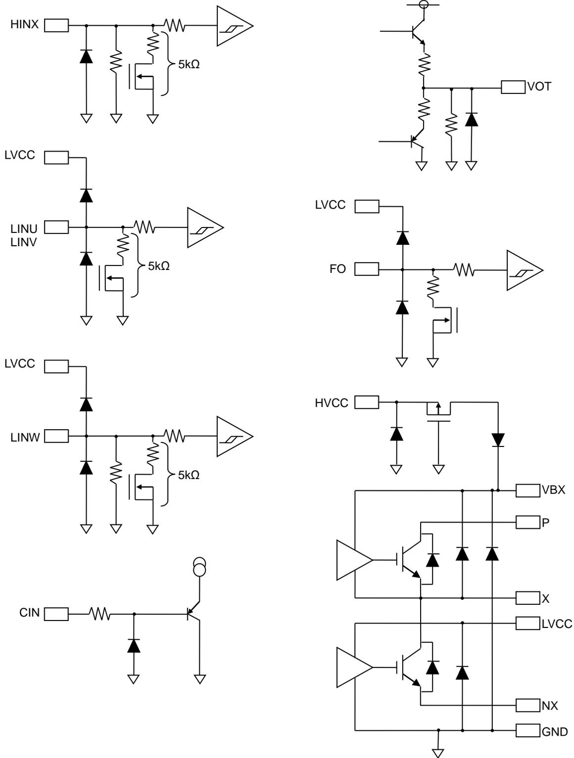
Figure 19. Input / Output Equivalent Circuit (X=U, V, W)
