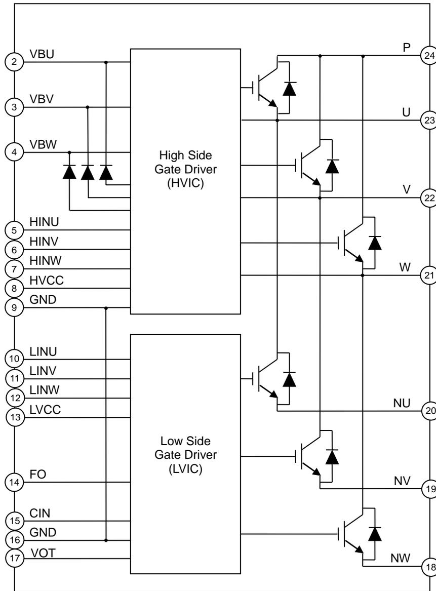
Figure 3. Block Diagram
