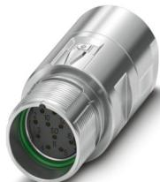
M23, Coupler connector, series: M23 PRO, straight, shielded: yes, for standard and ONECLICK fast locking system, No. of pos.: 12, Direction of rotation: Counter direction, contact connection type: Socket, Crimp connection, cable diameter range: 3 mm ... 15 mm, coding: N, Item is lead-free in accordance with RoHS II without Exemption 6c (Pb < 0.1 %)
