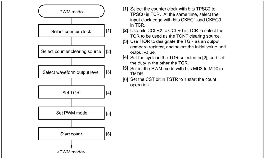
**Figure 8.20 Example of PWM Mode Setting Procedure**
