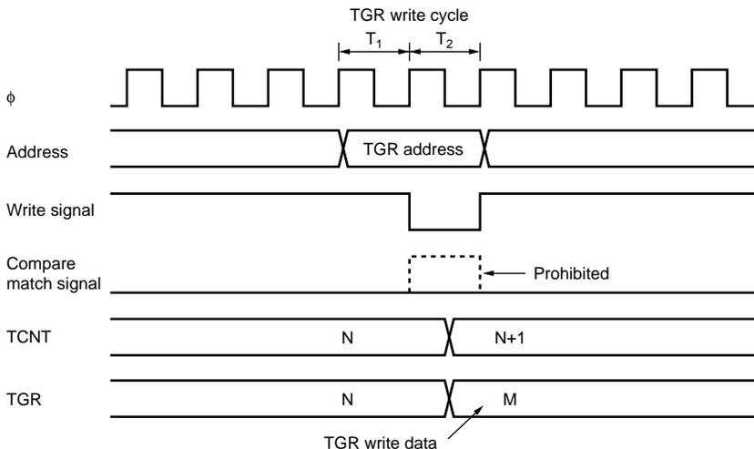
**Figure 8.46 Contention between TGR Write and Compare Match**
