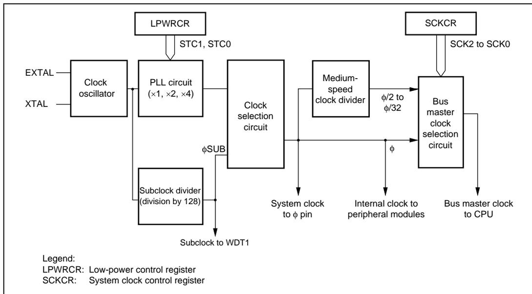
**Figure 15.1 Block Diagram of Clock Pulse Generator**
