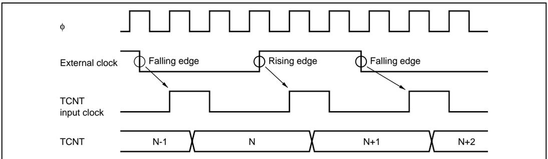
**Figure 8.31 Count Timing in External Clock Operation**
