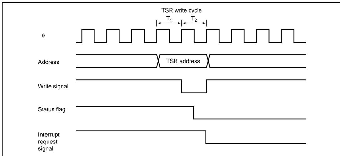
**Figure 8.42 Timing for Status Flag Clearing by CPU**
