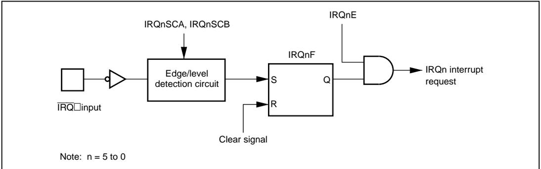
**Figure 5.2 Block Diagram of Interrupts IRQ0 to IRQ5**
