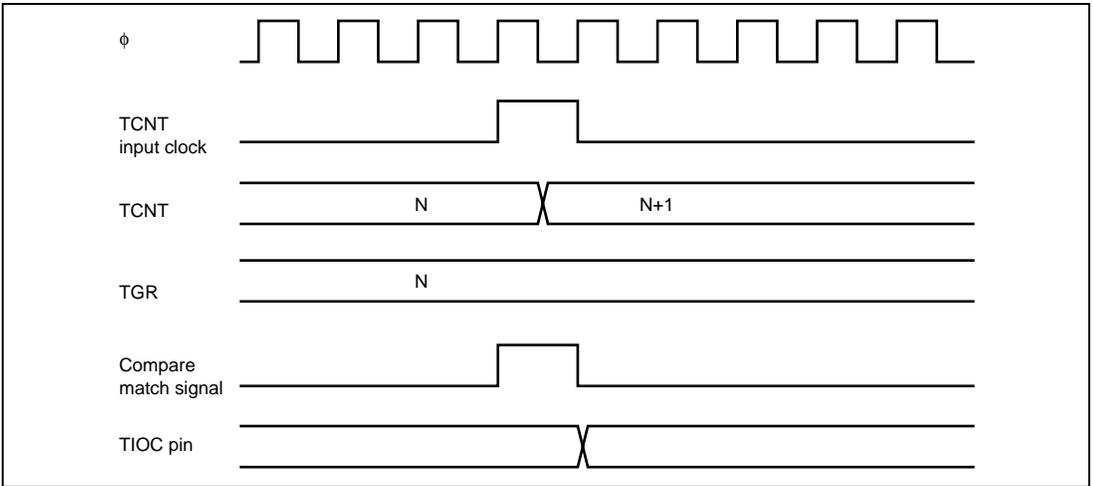
**Figure 8.32 Output Compare Output Timing**
