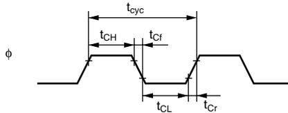
**Figure 18.2 System Clock Timing**
