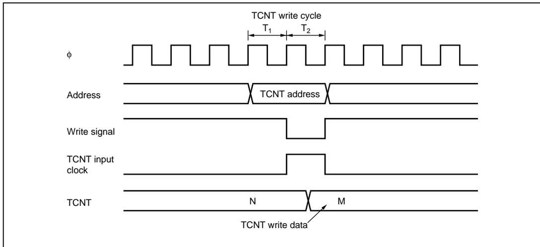
**Figure 8.45 Contention between TCNT Write and Increment Operations**
