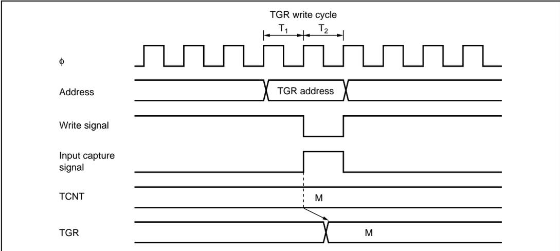
**Figure 8.49 Contention between TGR Write and Input Capture**
