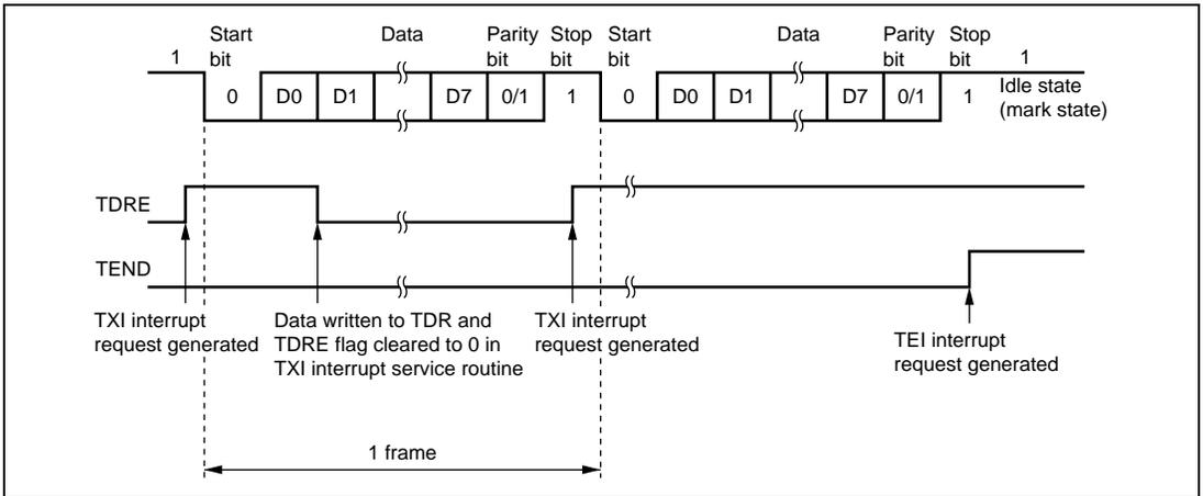
**Figure 10.6 Example of Operation in Transmission in Asynchronous Mode
