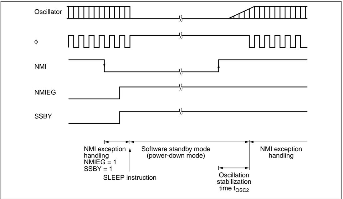
**Figure 16.3 Software Standby Mode Application Example**
