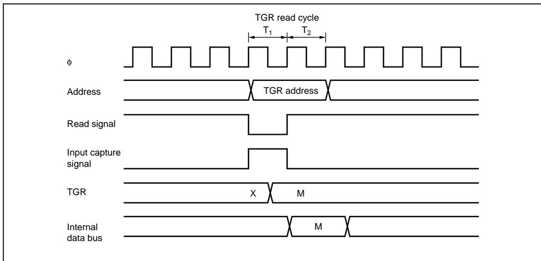
**Figure 8.48 Contention between TGR Read and Input Capture**
