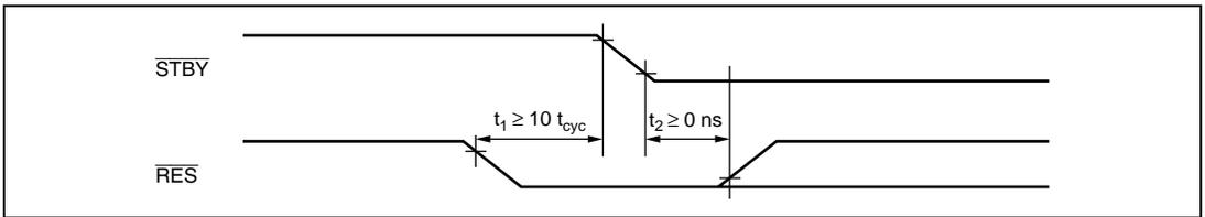
**Figure 16.4** Timing of Transition to Hardware Standby Mode
