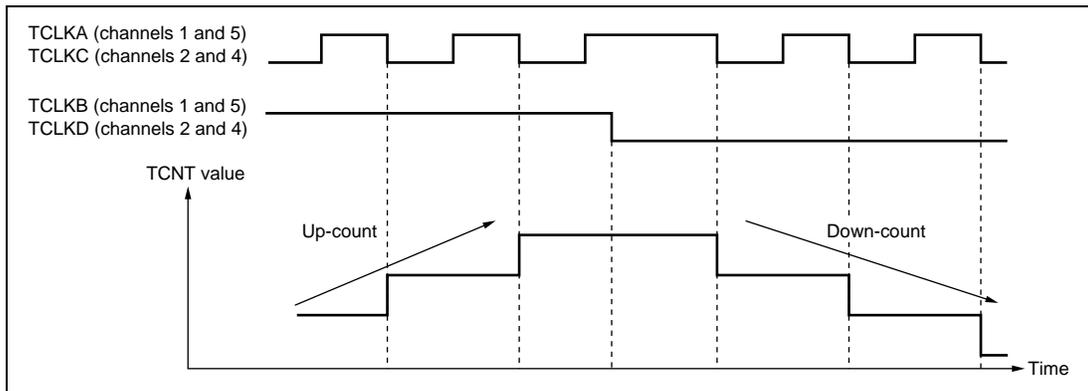
**Figure 8.26 Example of Phase Counting Mode 2 Operation**
