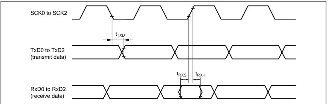
**Figure 18.10 SCI Input/Output Timing (Clocked Synchronous Mode)**
