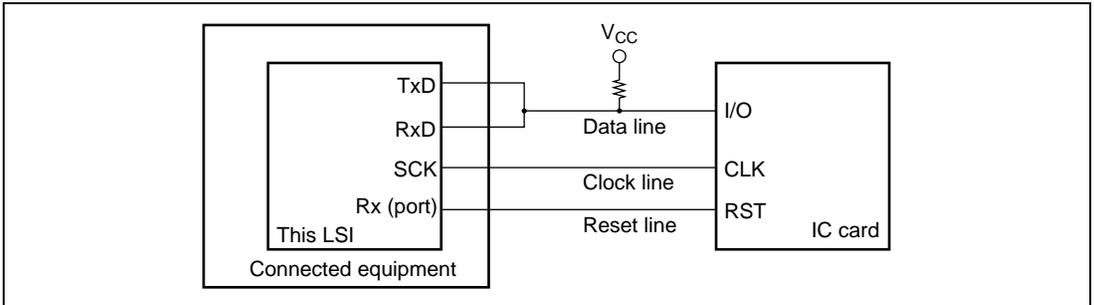
**Figure 10.21 Schematic Diagram of Smart Card Interface Pin Connections**
