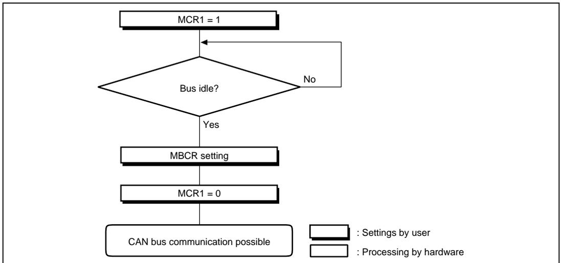
**Figure 11.14 HCAN Halt Mode Flowchart**
