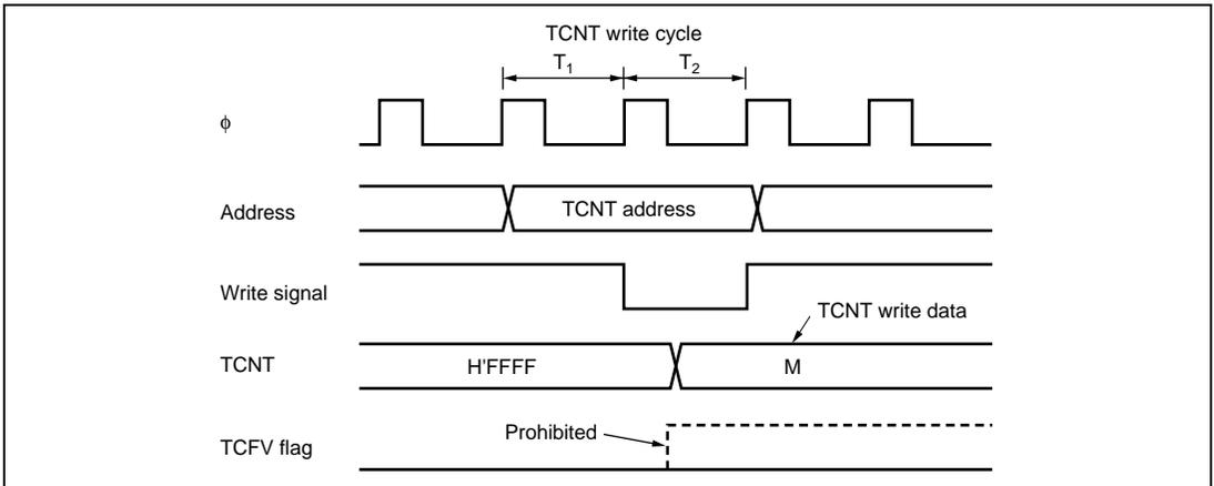
**Figure 8.52 Contention between TCNT Write and Overflow**
