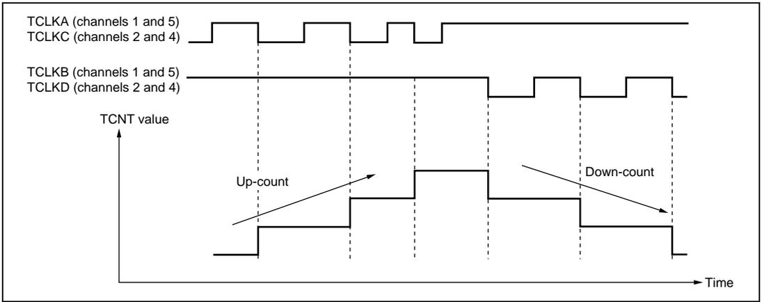
**Figure 8.27 Example of Phase Counting Mode 3 Operation**
