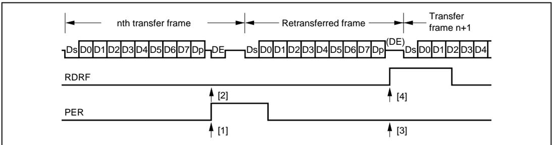
Figure 10.29 Retransfer Operation in SCI Receive Mode
