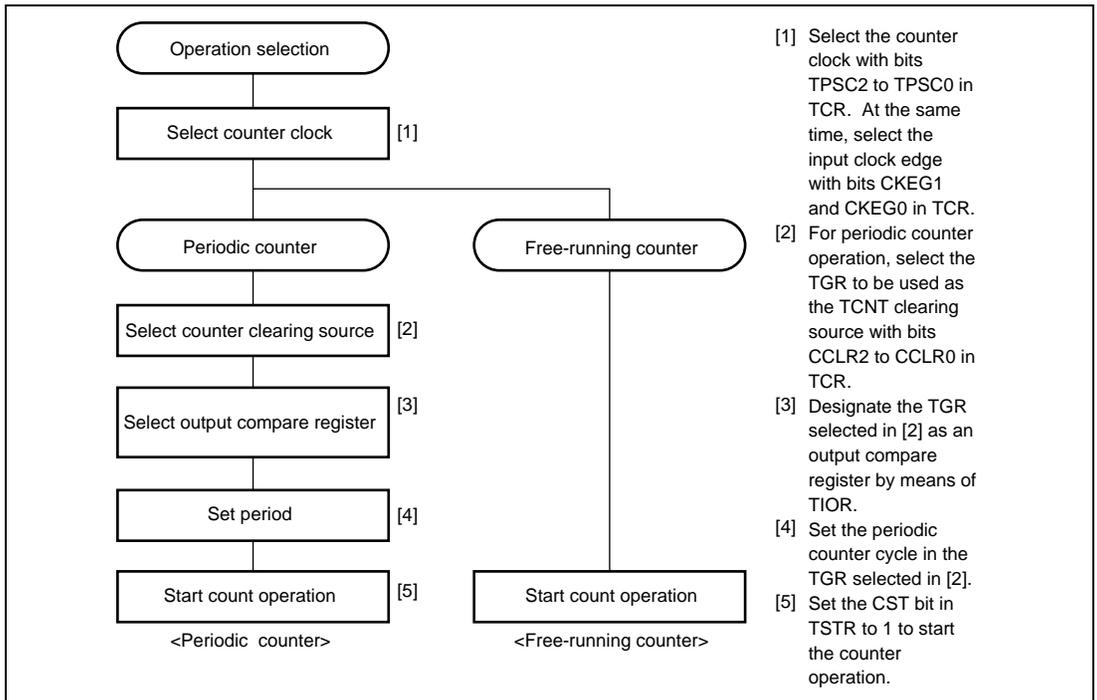
**Figure 8.2 Example of Counter Operation Setting Procedure**
