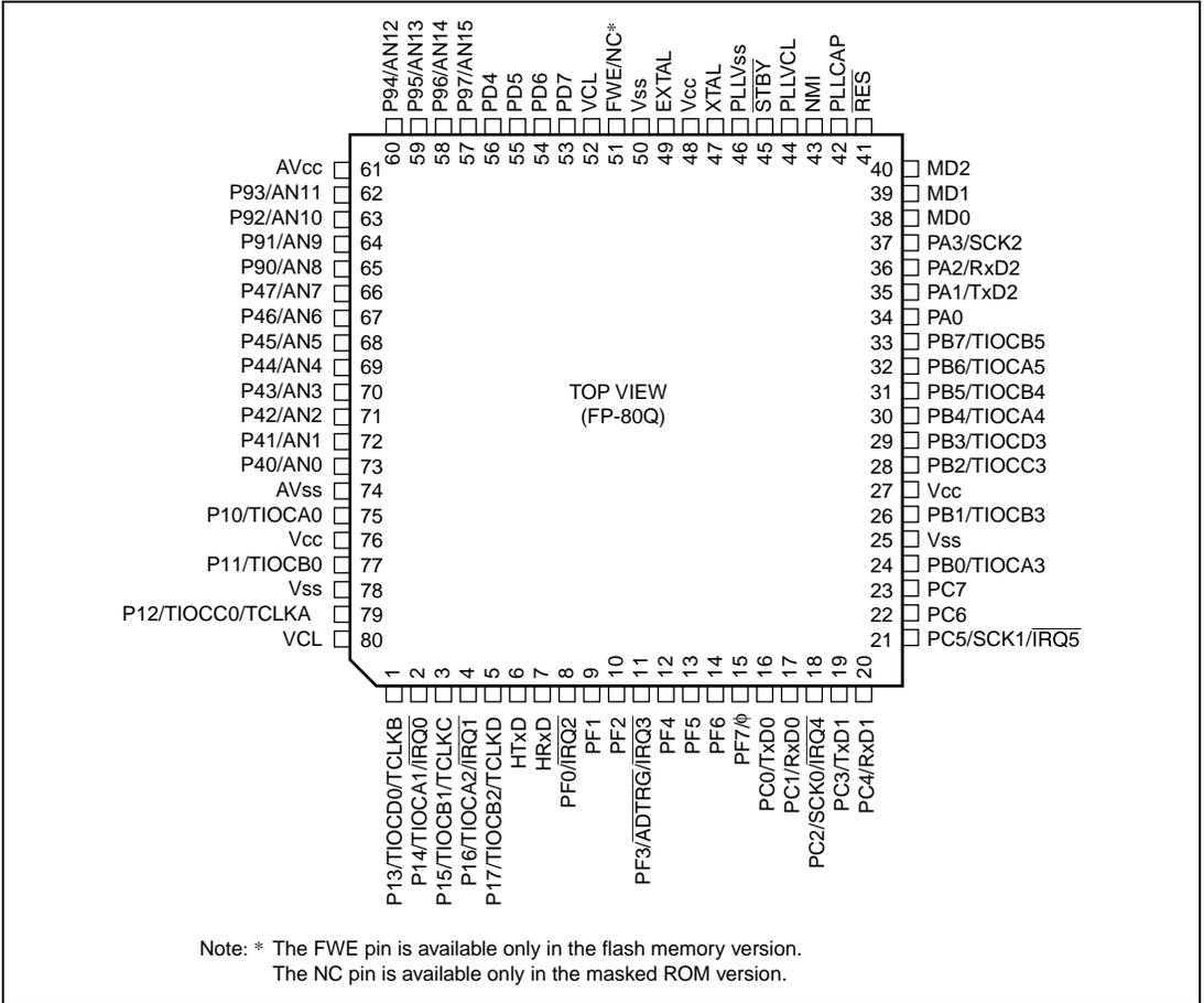
**Figure 1.2 Pin Arrangement**
