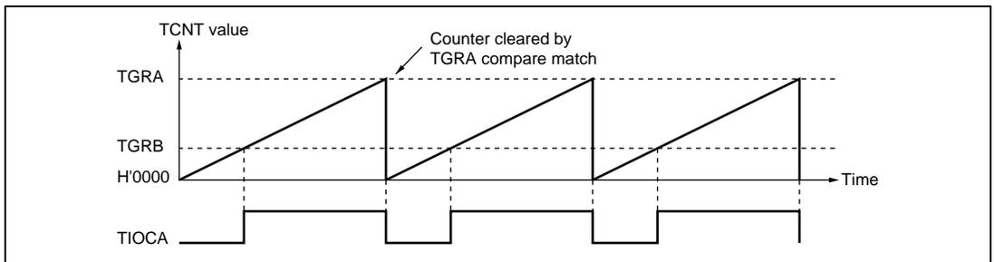
**Figure 8.21 Example of PWM Mode Operation (1)**
