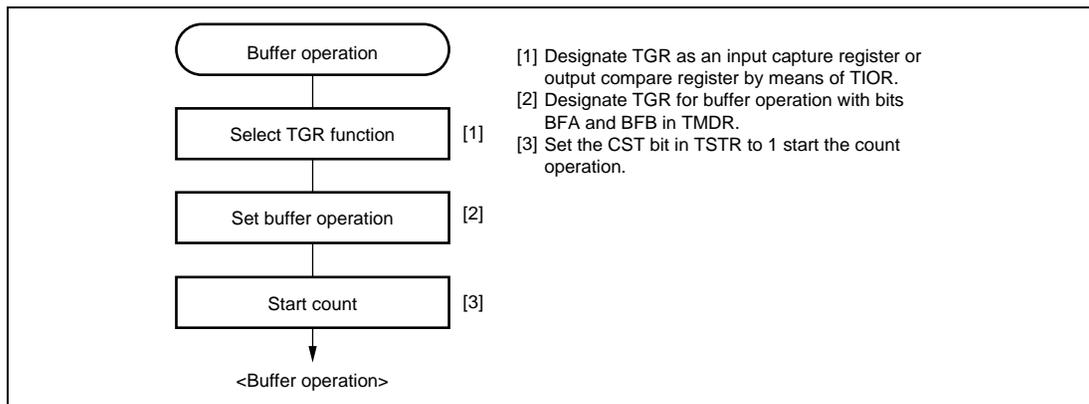
**Figure 8.14 Example of Buffer Operation Setting Procedure**
