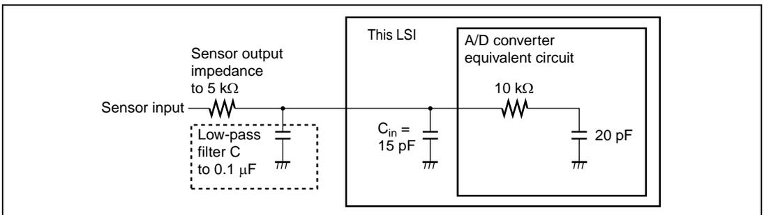
Figure 12.6 Example of Analog Input Circuit
