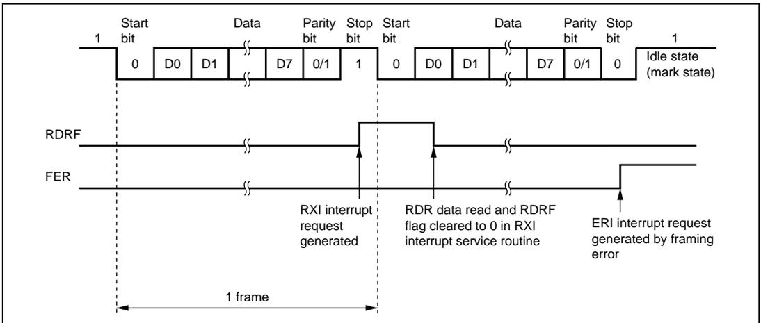
**Figure 10.8 Example of SCI Operation in Reception
