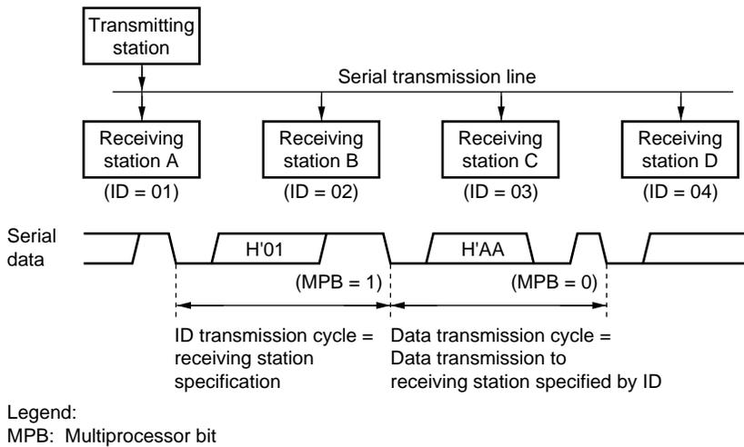
**Figure 10.10 Example of Communication Using Multiprocessor Format
