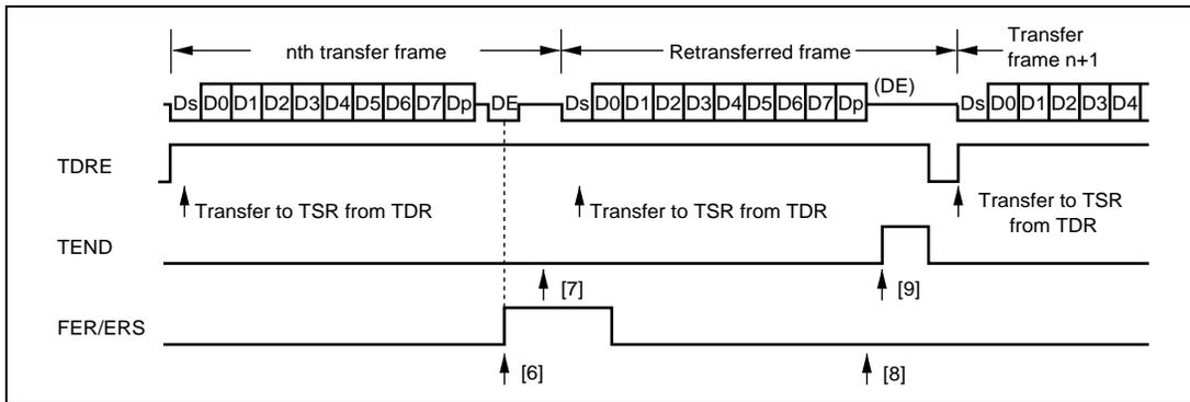
**Figure 10.26 Retransfer Operation in SCI Transmit Mode**
