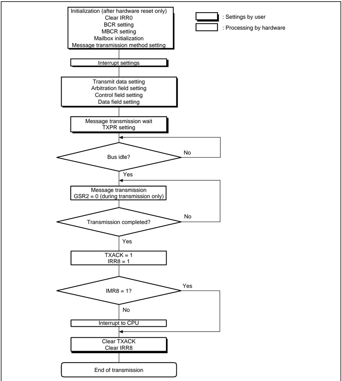
Figure 11.9 Transmission Flowchart
