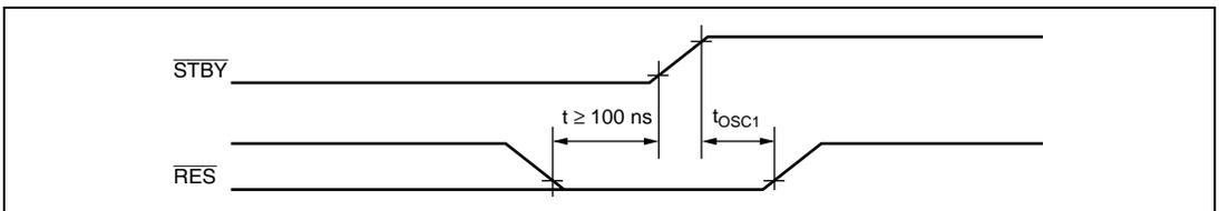
**Figure 16.5** Timing of Recovery from Hardware Standby Mode
