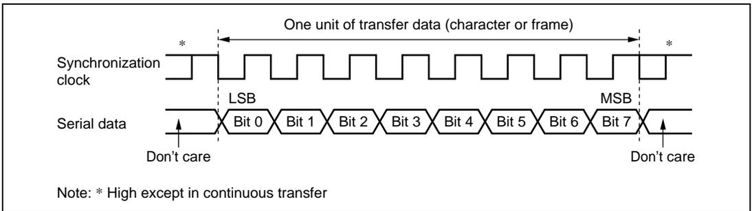
**Figure 10.14 Data Format in Synchronous Communication (For LSB-First)**
