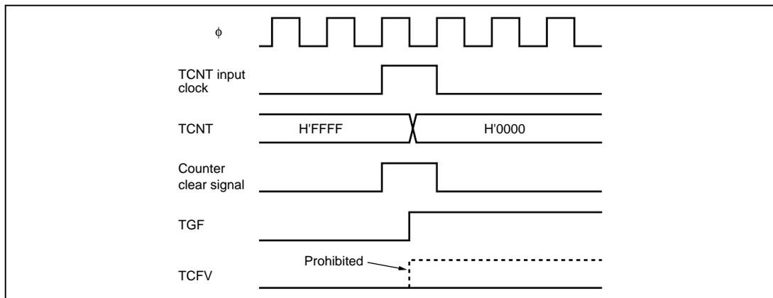
**Figure 8.51 Contention between Overflow and Counter Clearing**
