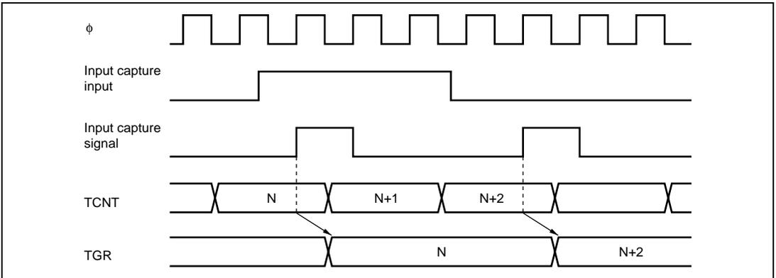
**Figure 8.33 Input Capture Input Signal Timing**
