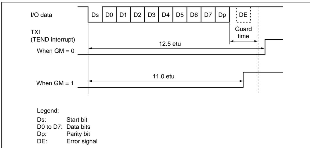
**Figure 10.27 TEND Flag Generation Timing in Transmission Operation**
