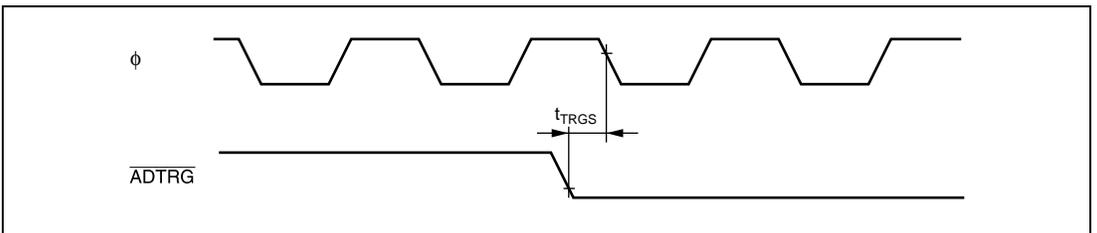
**Figure 18.11 A/D Converter External Trigger Input Timing**
