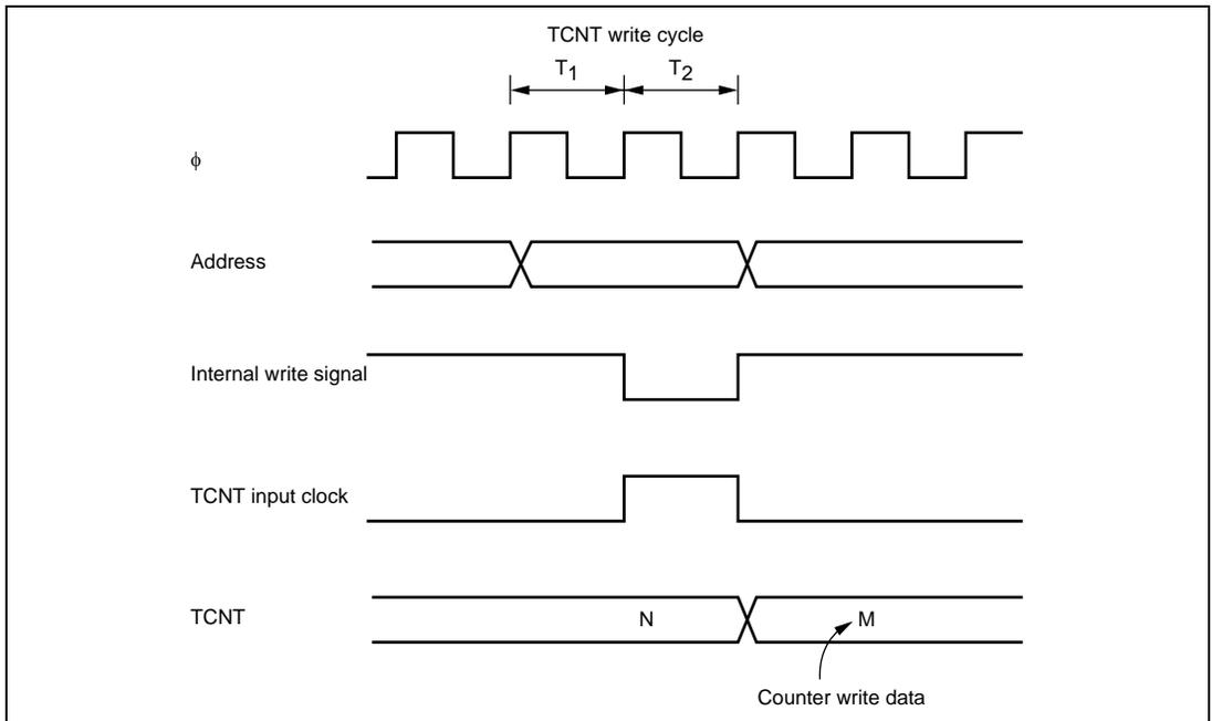
**Figure 9.6 Contention between TCNT Write and Increment**
