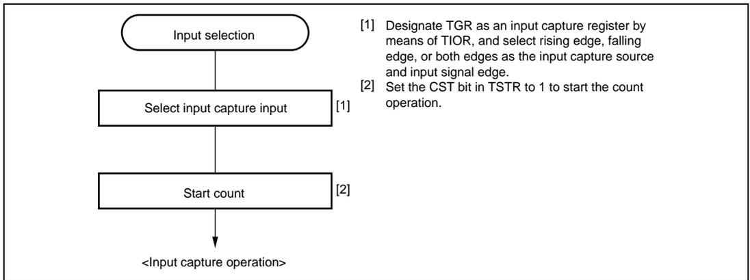
**Figure 8.8 Example of Input Capture Operation Setting Procedure**
