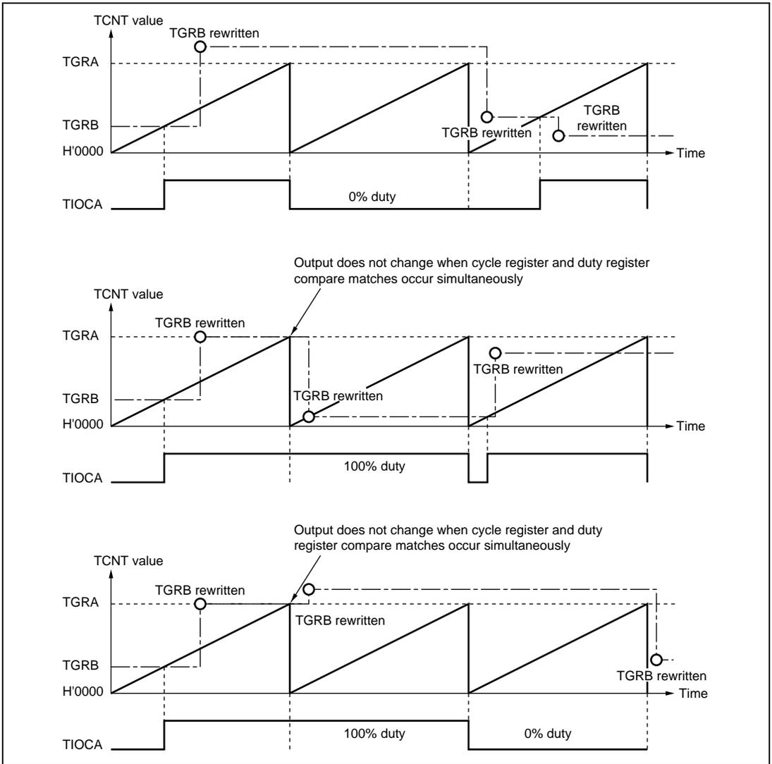
**Figure 8.23 Example of PWM Mode Operation (3)**
