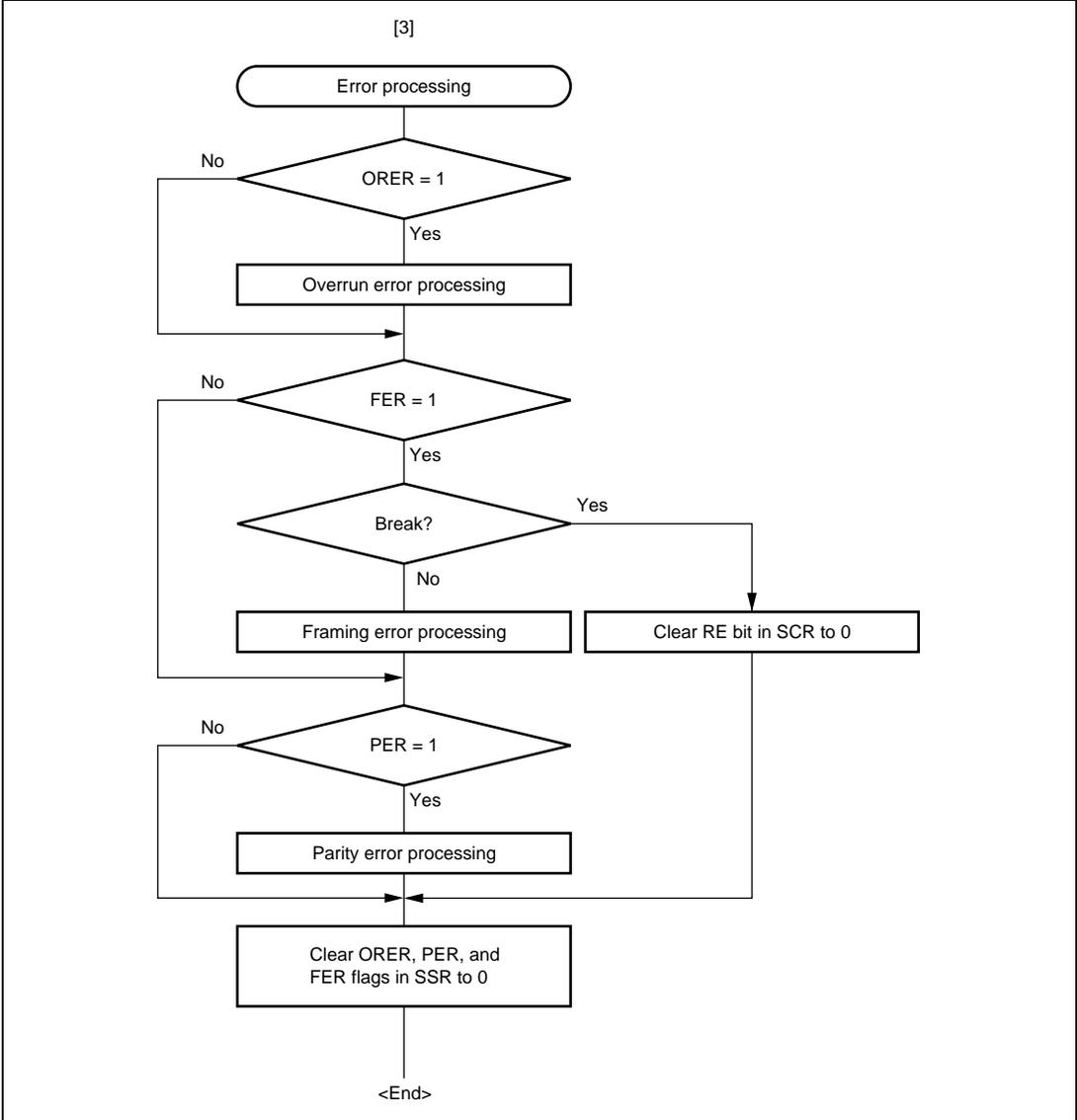
**Figure 10.9 Sample Serial Reception Data Flowchart (2)**
