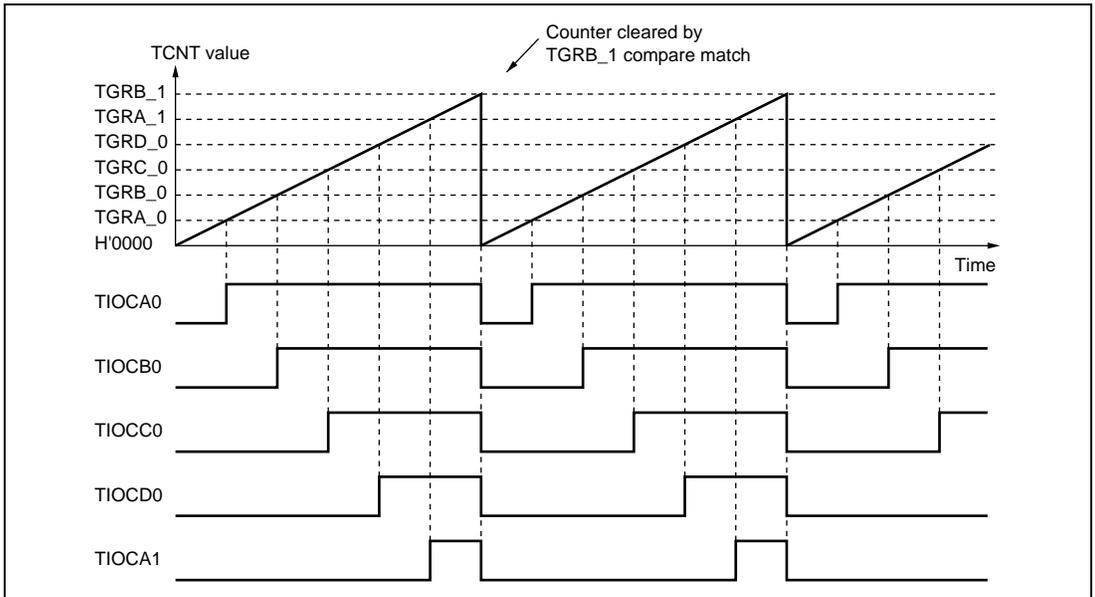
**Figure 8.22 Example of PWM Mode Operation (2)**
