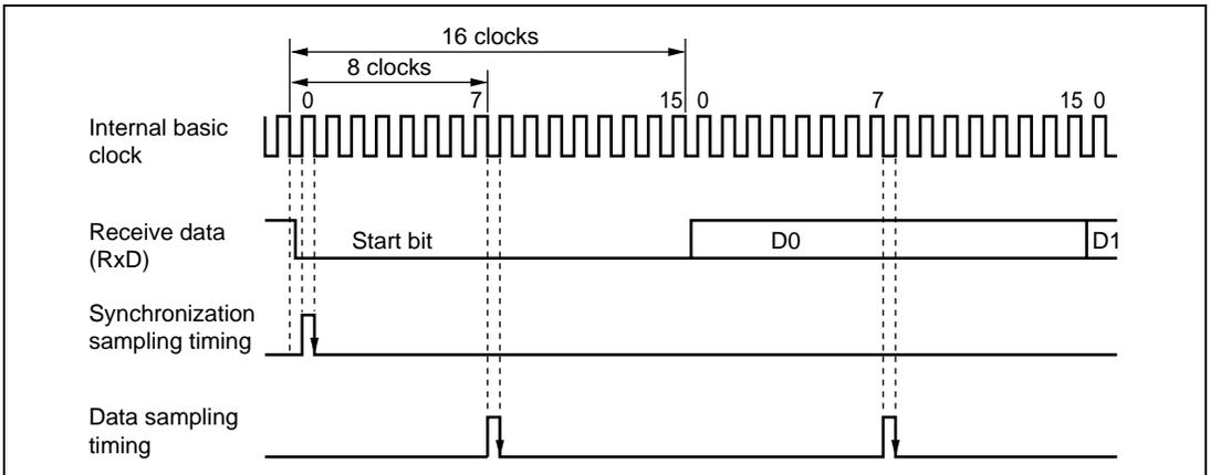
Figure 10.3 Receive Data Sampling Timing in Asynchronous Mode
