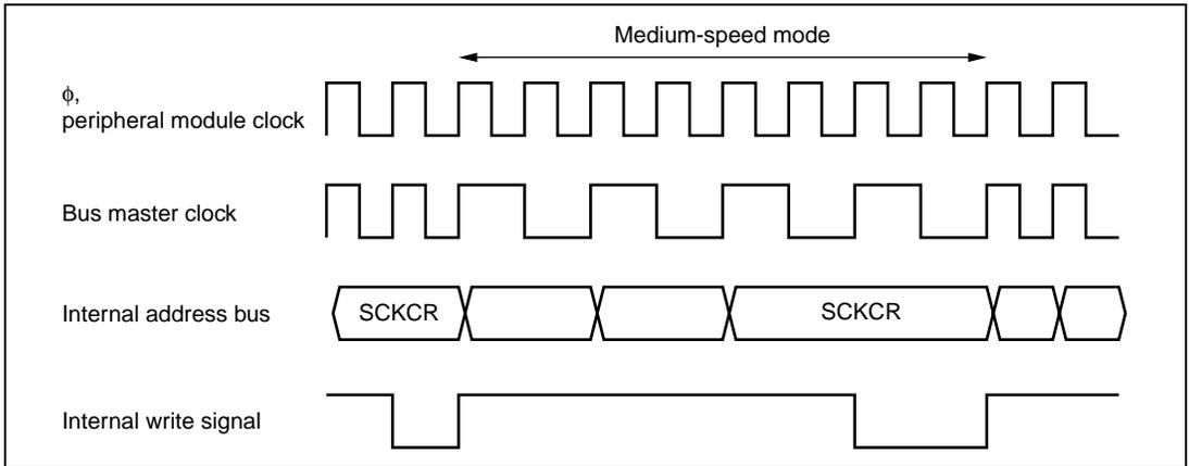
**Figure 16.2 Medium-Speed Mode Transition and Clearance Timing**
