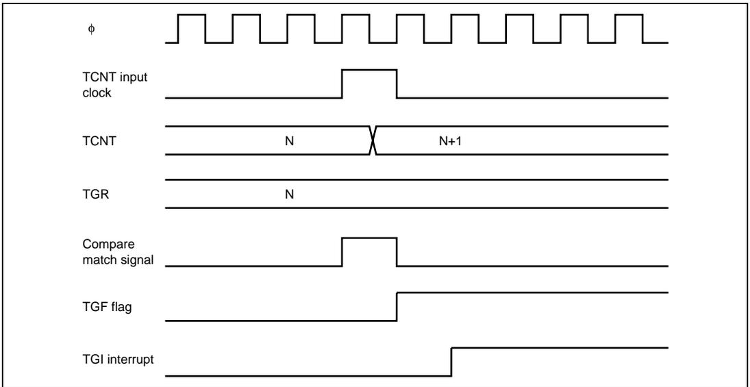
**Figure 8.38 TGI Interrupt Timing (Compare Match)**
