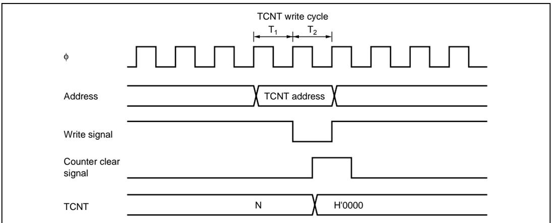
**Figure 8.44 Contention between TCNT Write and Clear Operations**
