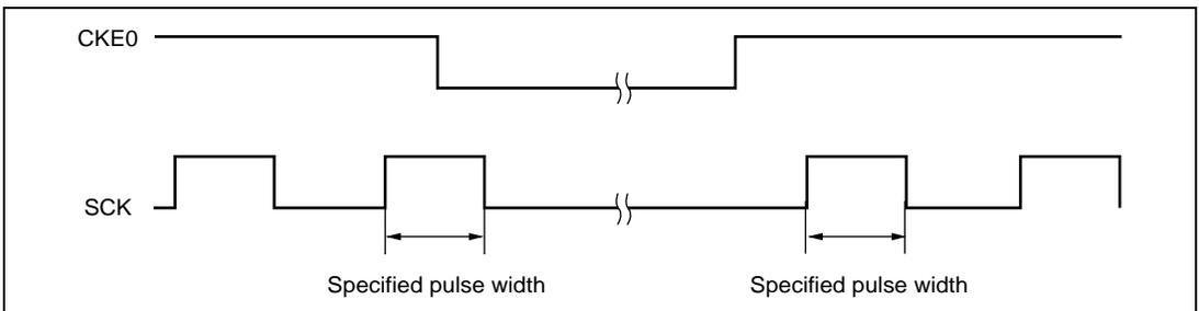
**Figure 10.31 Timing for Fixing Clock Output Level**
