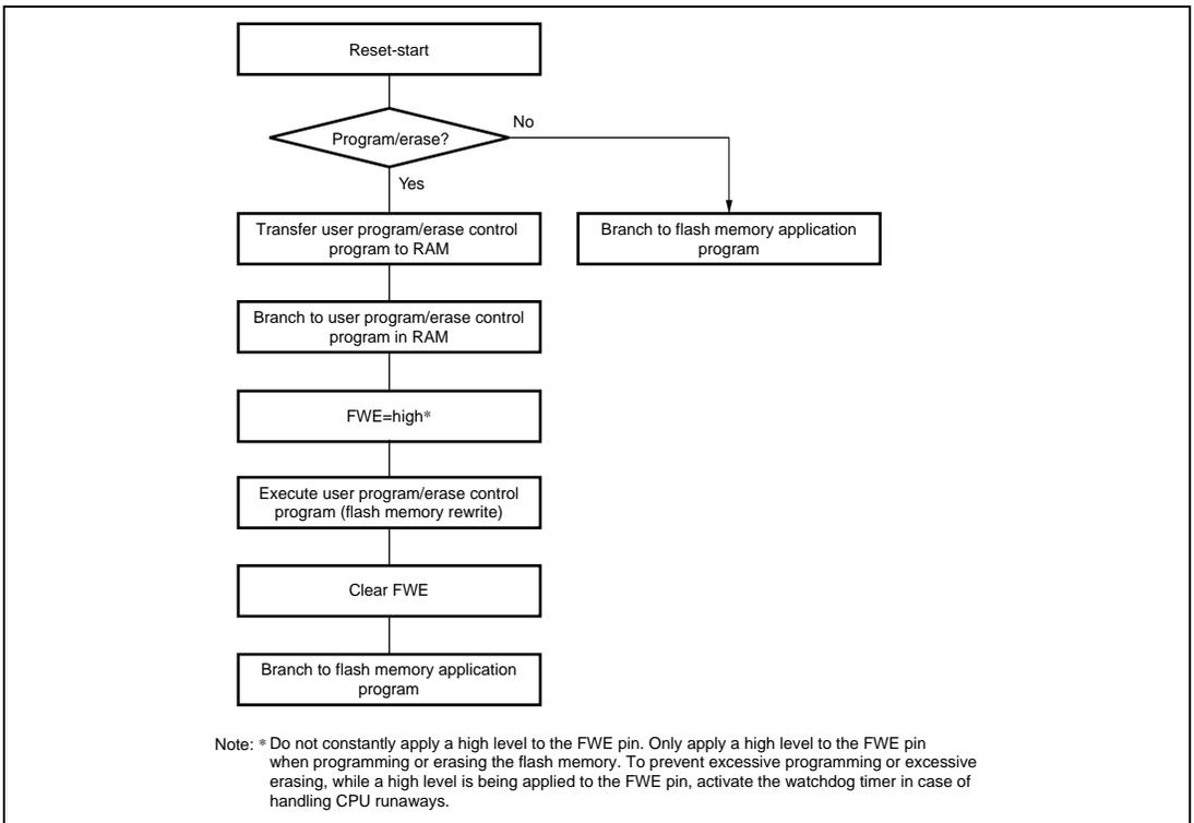
**Figure 14.6 Programming/Erasing Flowchart Example in User Program Mode**
