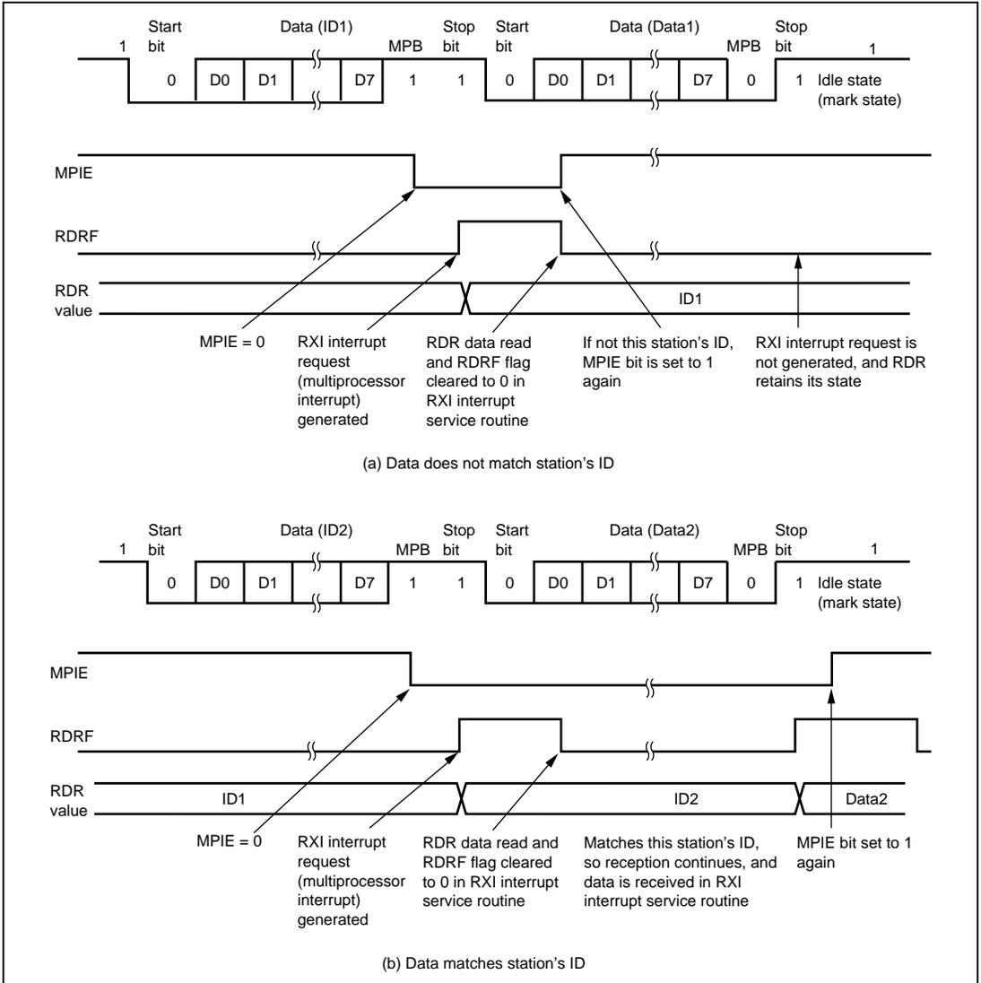
**Figure 10.12 Example of SCI Operation in Reception
