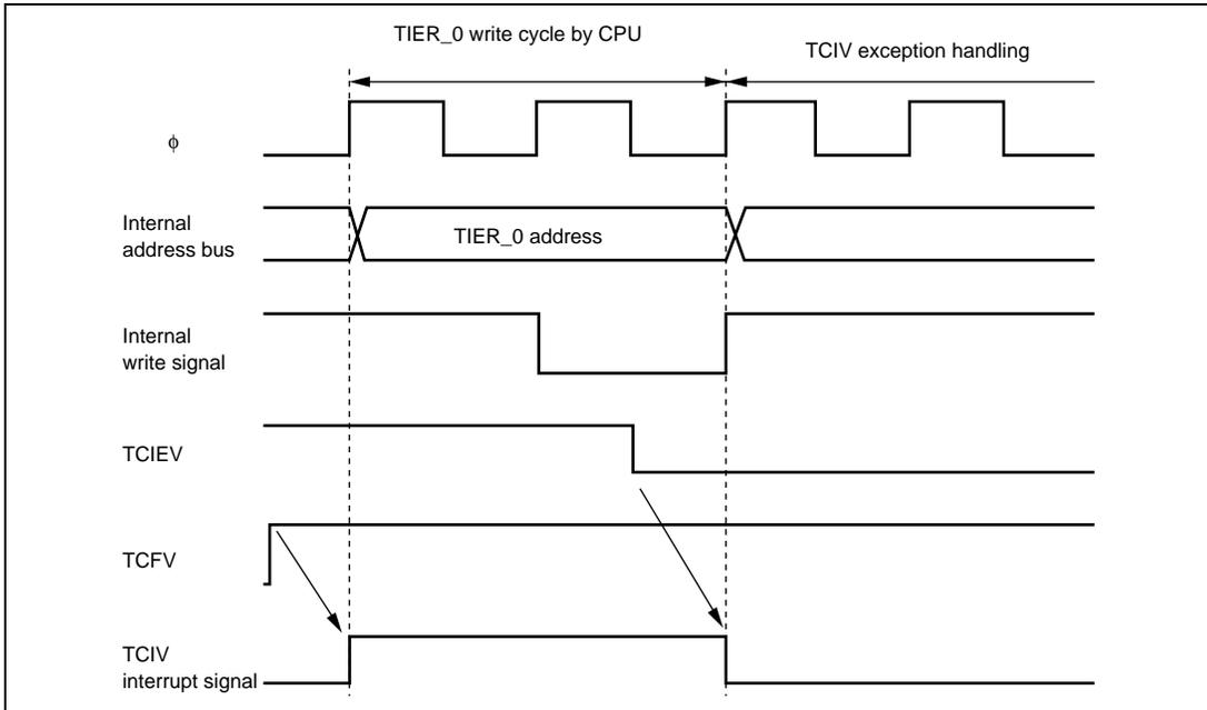
**Figure 5.6 Contention between Interrupt Generation and Disabling**
