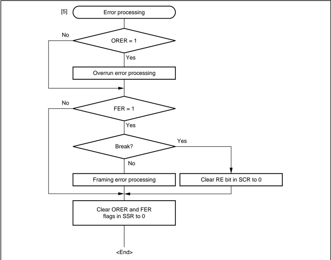
**Figure 10.13 Sample Multiprocessor Serial Reception Flowchart (2)**
