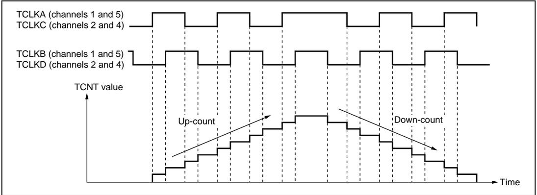
**Figure 8.25 Example of Phase Counting Mode 1 Operation**
