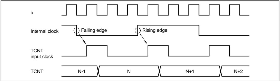
**Figure 8.30 Count Timing in Internal Clock Operation**
