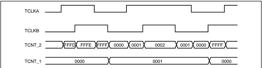
**Figure 8.19 Example of Cascaded Operation (2)**
