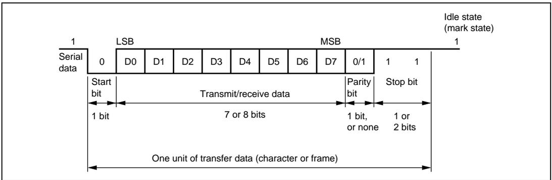
**Figure 10.2 Data Format in Asynchronous Communication
