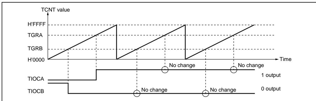
**Figure 8.6 Example of 0 Output/1 Output Operation**
