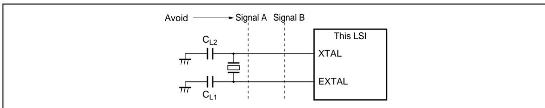
**Figure 15.6 Note on Board Design of Oscillator Circuit**
