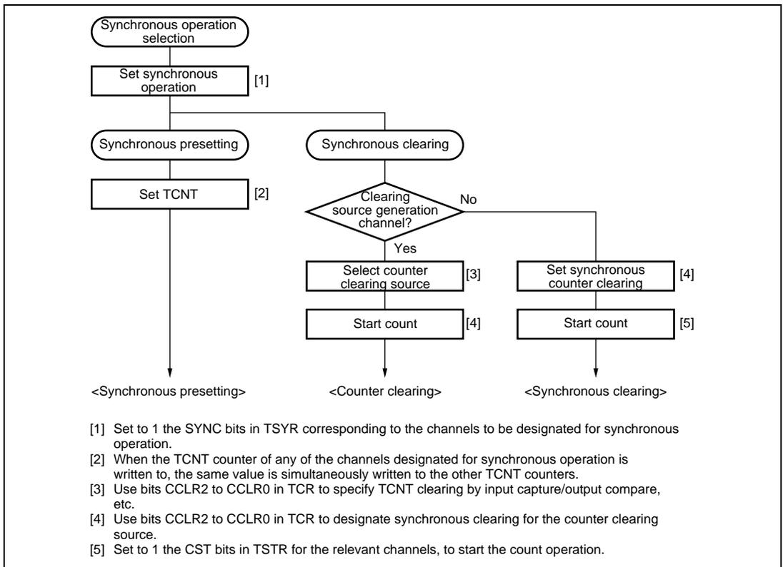
**Figure 8.10 Example of Synchronous Operation Setting Procedure**
