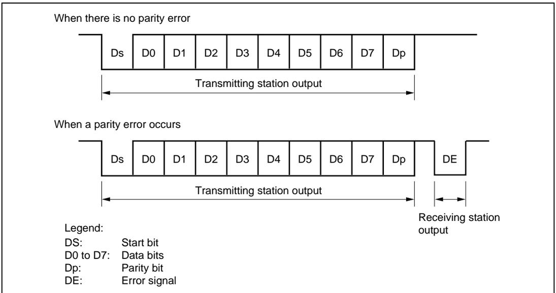
**Figure 10.22 Normal Smart Card Interface Data Format**
