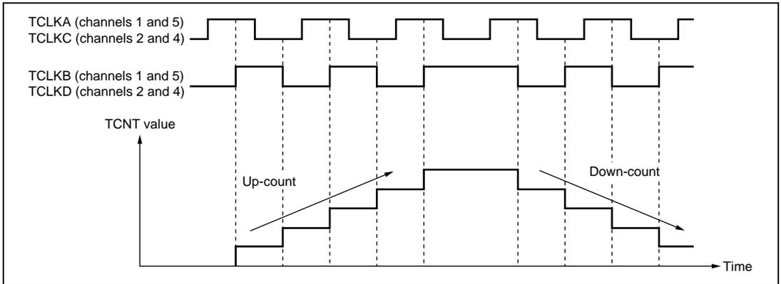
**Figure 8.28 Example of Phase Counting Mode 4 Operation**
