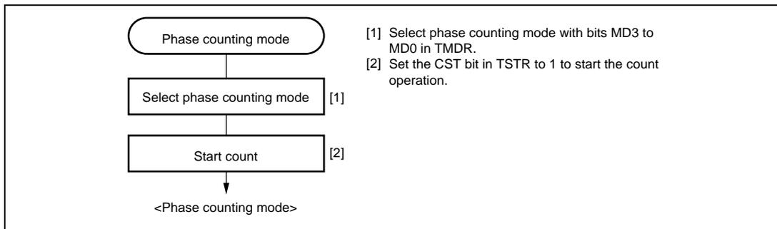
**Figure 8.24 Example of Phase Counting Mode Setting Procedure**
