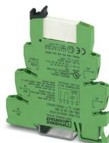
PLC-INTERFACE, consisting of DIN rail-mountable basic terminal block with screw connection and plug-in miniature relay with power contact, 1 changeover contact, input voltage: 120 V AC/110 V DC, UL/cUL: approved for use in Ex Zone Class I, Div. 2 and ATEX (Zone 2)
