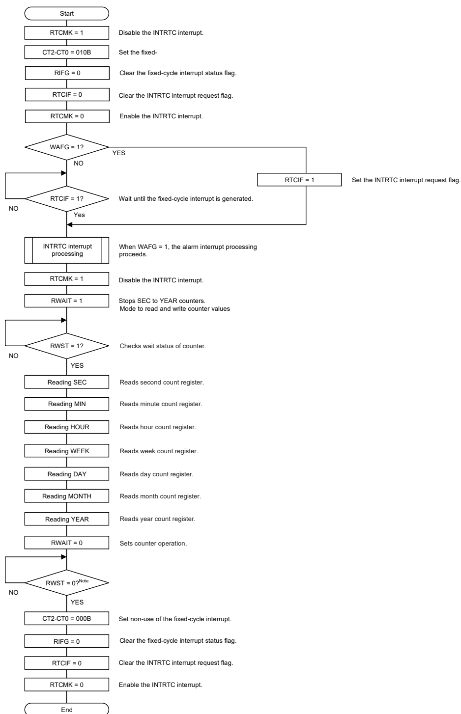
Figure 7-22. Procedure for Reading Real-time Clock (When the Alarm Interrupt is in Use)
