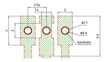
Cu area appr. 8mm² per pad and side with solder resist
