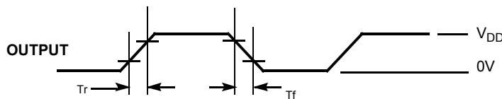
Output Rise time (Tr) =  $(0.6 \times V_{DD})/SR1$  (or SR3)
