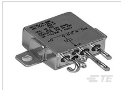
Relay & Contactor Type: **General Purpose Power Relay**Coil Magnetic System: **Polarized, Monostable**Contact Arrangement: **1 Form C SPDT-CO**Current Type: **DC**Contact Current Rating: **25 A**
