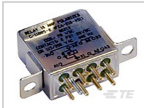
Relay & Contactor Type: **General Purpose Power Relay**Coil Magnetic System: **Polarized, Monostable**Contact Arrangement: **2 Form C DPDT-CO**Current Type: **AC**Contact Current Rating: **10 A**
