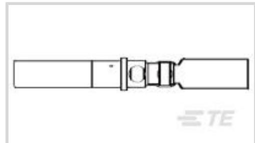
Compatible With Wire & Cable Type: **TwinAxial**Contact Type: **Socket**Contact Size: **Size 8**Wire Size: **20 AWG**
