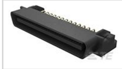
PCB Connector Assembly Type: **PCB Mount Header**PCB Mount Orientation: **Right Angle**Connector System: **Board-to-Board**Number of Positions: **30**Centerline (Pitch): **1.27 mm [.05 in]**
