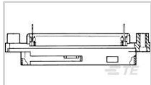
Connector & Housing Type: **Plug**Connector System: **Cable-to-Board**Number of Positions: **24**Centerline (Pitch): **2.16 mm [.085 in]**Number of Rows: **2**[All D-Sub Plug Assembly: Vertical, 2.16mm \(4\)](#)**Features****Product Type Features**
