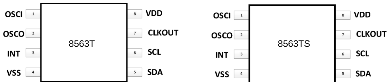
Figure 2. Pin configuration for PCF8563
