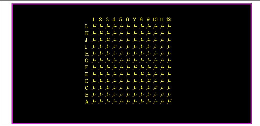
Figure 8: LED Board Component Placement Guide - Top Layer
