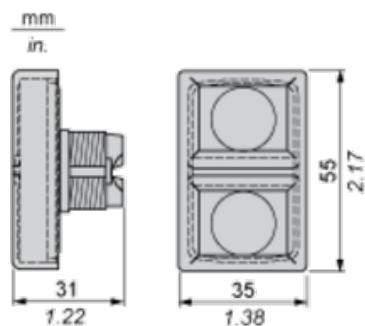
Panel Cut-out for Pushbuttons, Switches and Pilot Lights (Finished Holes, Ready for Installation)
