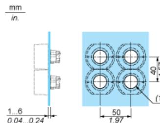
(1) Ø22.5 mm recommended ( $\varnothing 22.3_0^{+0.4}$ ) / Ø0.89 in. recommended ( $\varnothing 0.88_0^{+0.016}$ )
