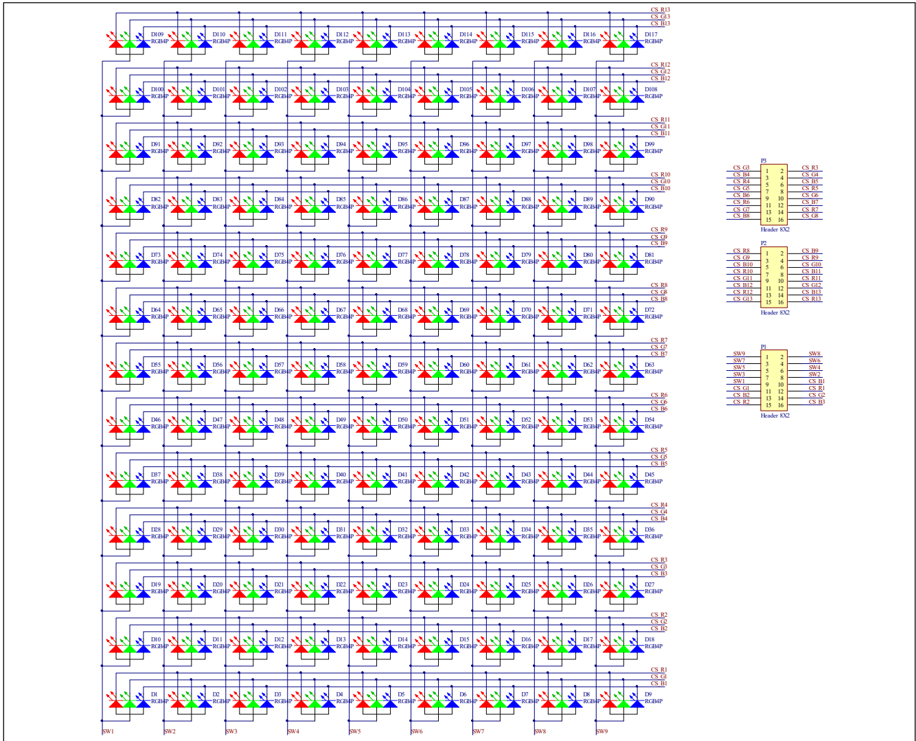
Figure 4: FxLED_9x13_ARRAY Application Schematic
