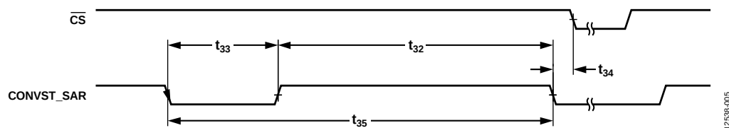
Figure 5. SAR ADC Timing Diagram
