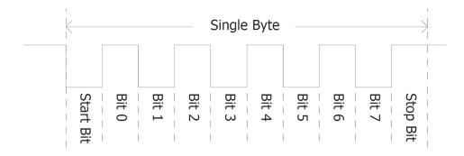
uLCD-70D Series Serial Ports - TTL Level
