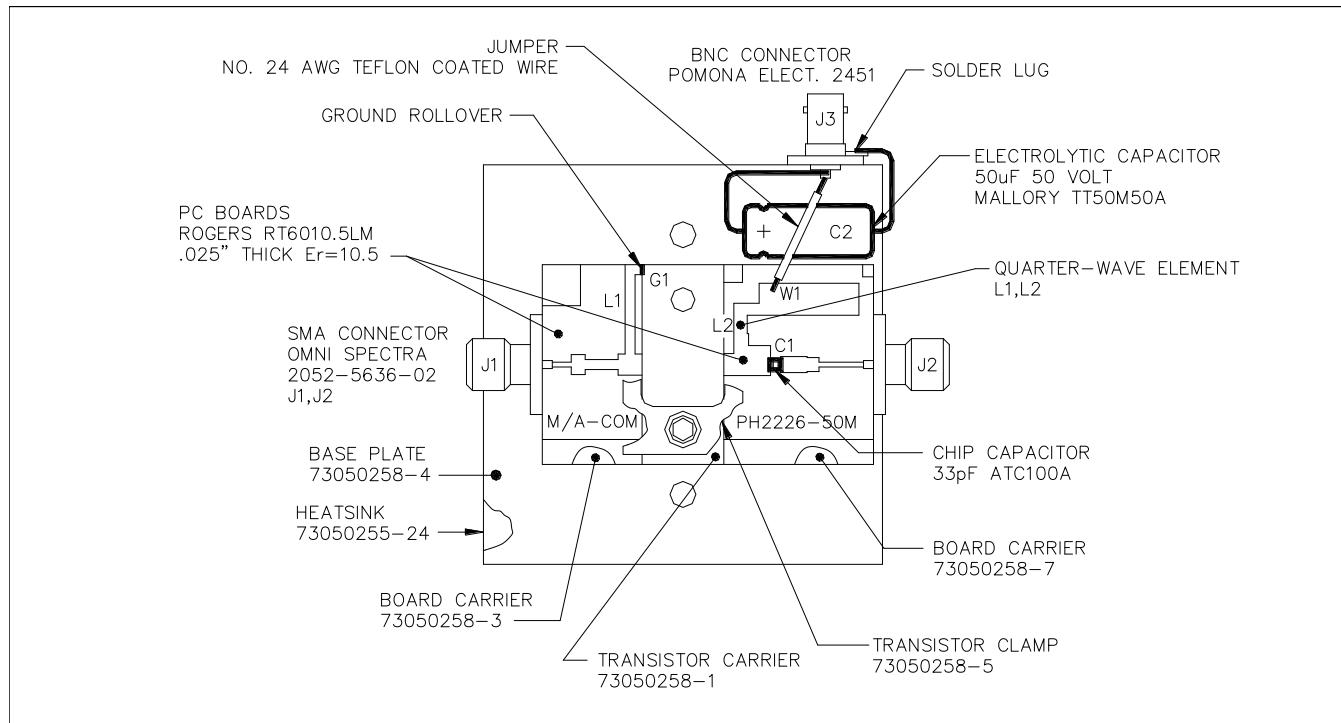
**Radar Pulsed Power Transistor
