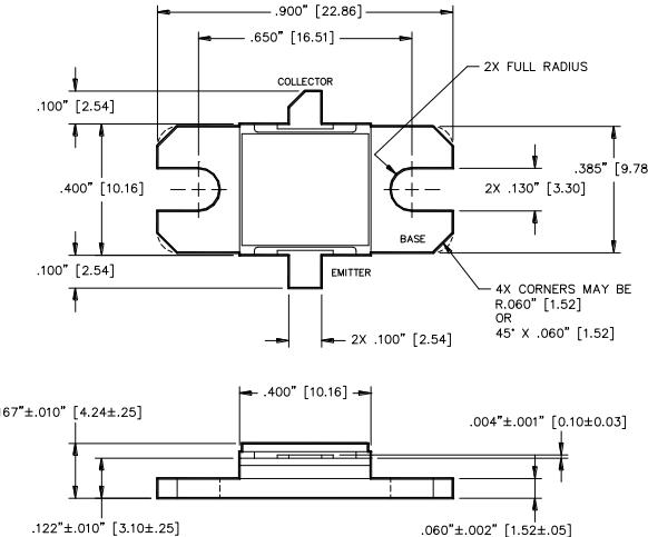
UNLESS OTHERWISE NOTED, TOLERANCES ARE INCHES  $\pm .005$  [MILLIMETERS  $\pm 0.13$ MM]
