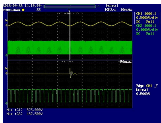
Figure 148 – (+) 2.5 kV Ring Wave Surge, 270° Phase Angle. Lower: V_{DRAIN} , 100 V / div., 10 ms / div. Peak V_{DRAIN} : 437.50 V.
